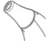
Keep the protective cap snapped onto the top of the thermometer when not in use to protect the tip from damage.
