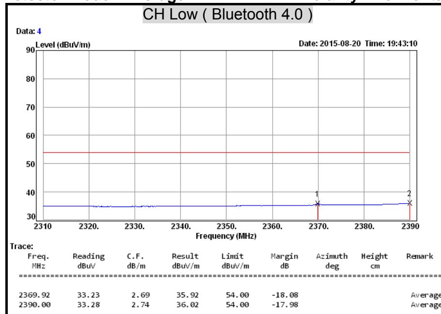
**Detector Mode : Peak****Polarity : Vertical****CH Low ( Bluetooth 4.0 )**
