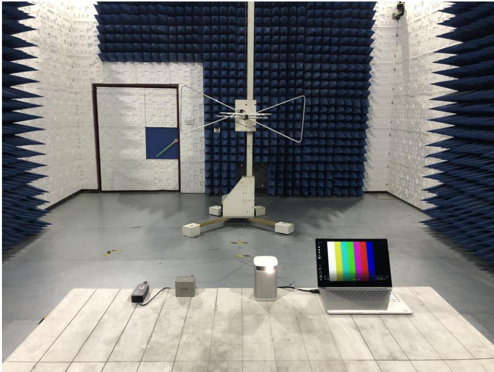
RADIATED EMISSION TEST SETUP ABOVE 1GHZ
