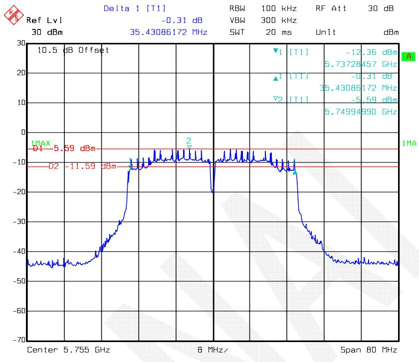
**802.11ac40 mode, 6 dB Bandwidth-5795 MHz, Antenna 1**
