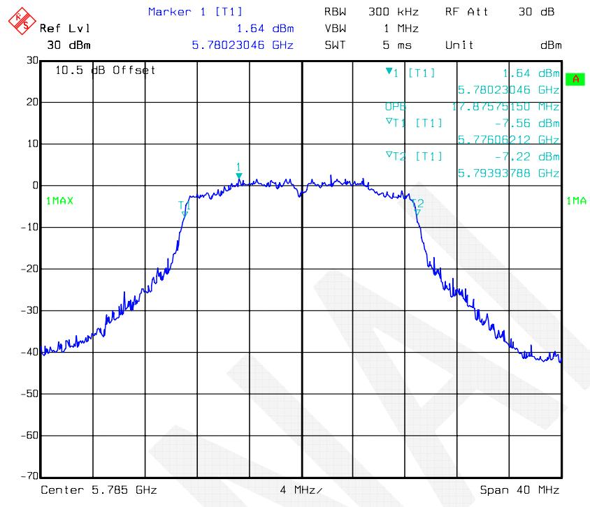
**802.11n-HT20 mode, 99% Occupied Bandwidth-5825 MHz, Antenna 2**
