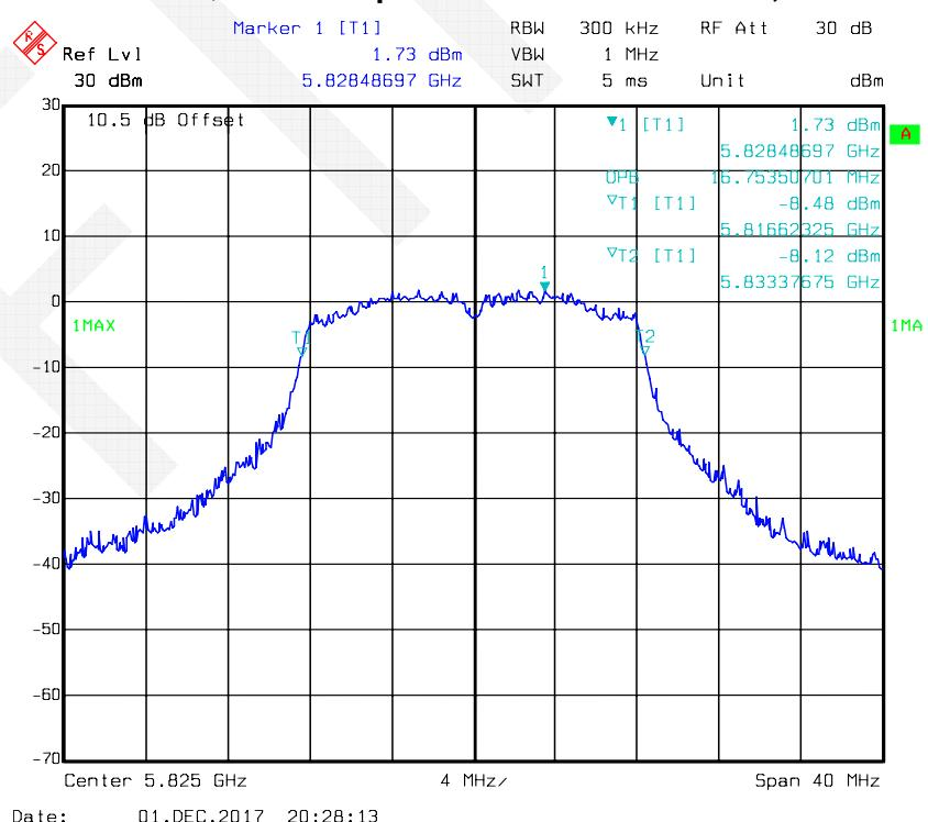
**802.11n-HT20 mode, 99% Occupied Bandwidth-5745 MHz, Antenna 1**
