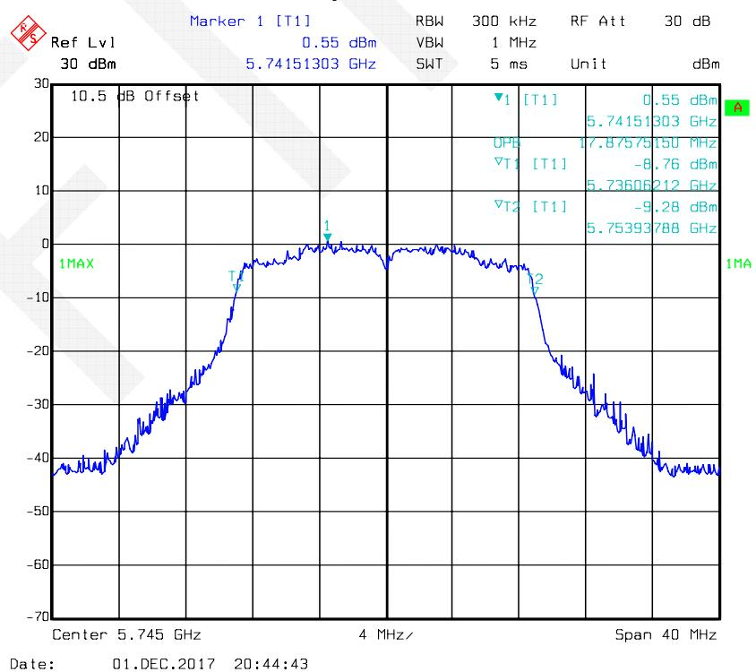
**802.11ac20 mode, 99% Occupied Bandwidth-5785 MHz, Antenna 2**
