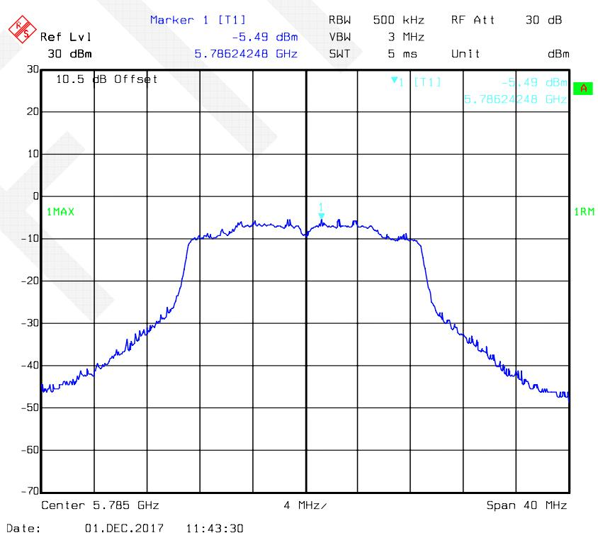
**802.11n-HT20 mode, Power Spectral Density-5825 MHz, Antenna 1**
