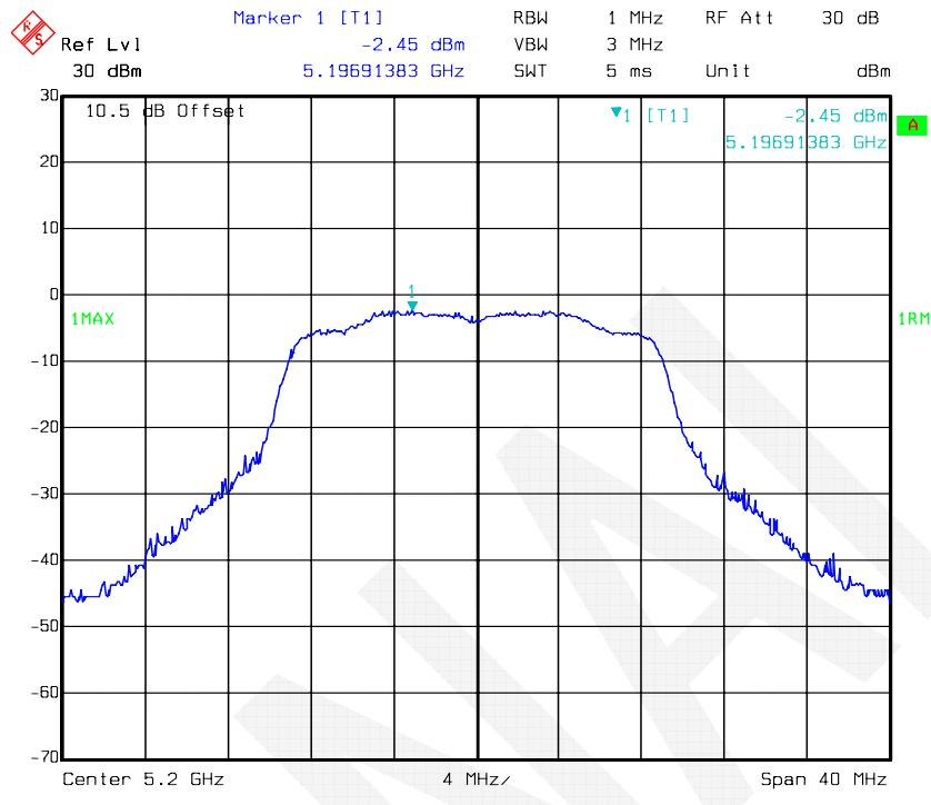
**802.11n-HT20 mode, Power Spectral Density-5240 MHz, Antenna 2**
