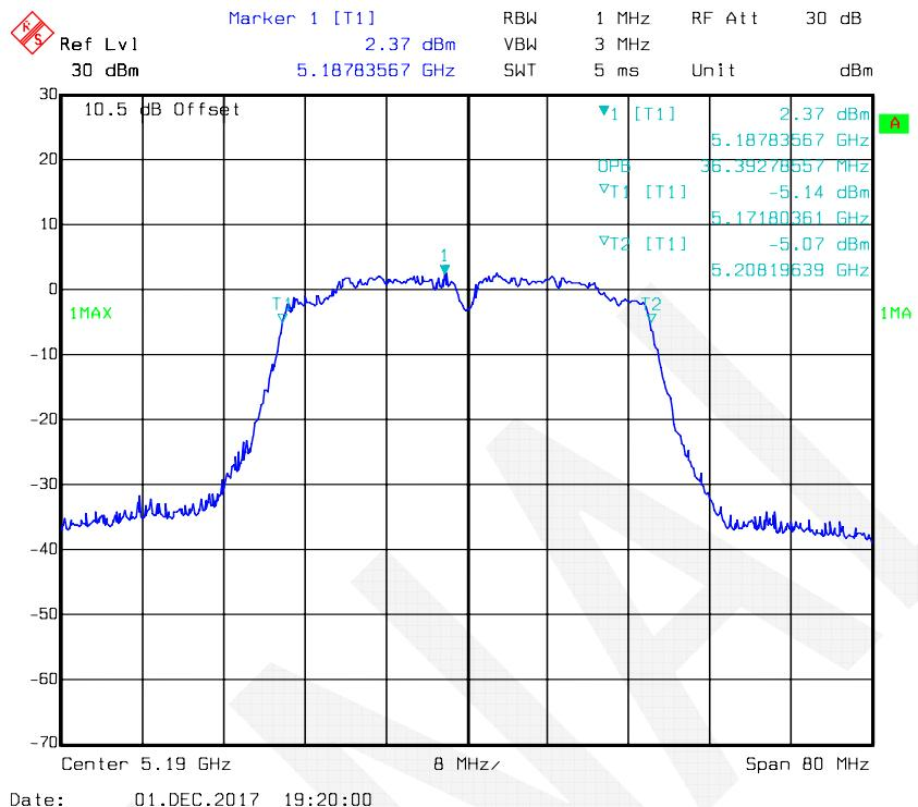
**802.11n-HT40 mode, 99% Occupied Bandwidth-5230 MHz, Antenna 1**
