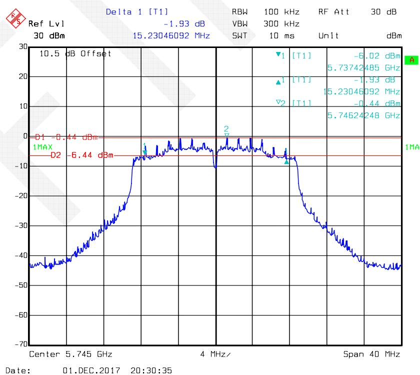
**802.11n-HT20 mode, 6 dB Bandwidth-5785 MHz, Antenna 2**
