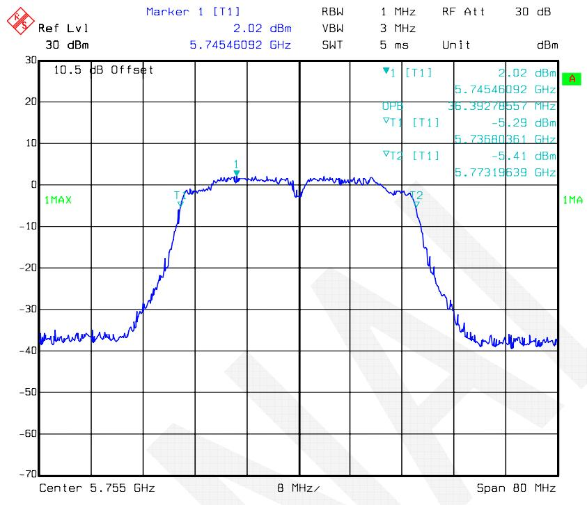
**802.11ac40 mode, 99% Occupied Bandwidth-5795 MHz, Antenna 2**
