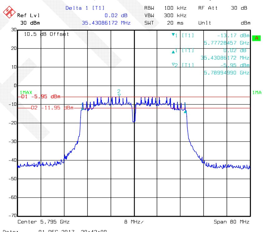
**802.11ac20 mode, 6 dB Bandwidth-5745 MHz, Antenna 1**
