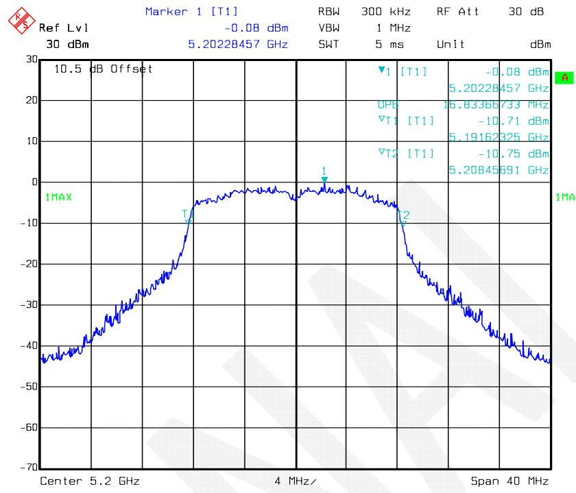
**802.11a mode, 99% Occupied Bandwidth -5240 MHz, Antenna 2**
