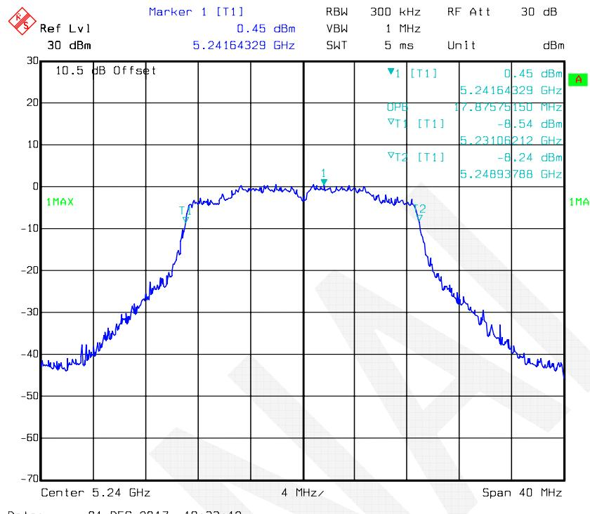
**802.11ac20 mode, 99% Occupied Bandwidth-5180 MHz, Antenna 2**
