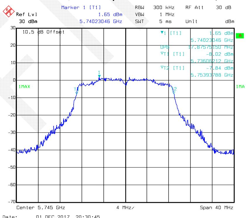
**802.11n-HT20 mode, 99% Occupied Bandwidth-5785 MHz, Antenna 2**
