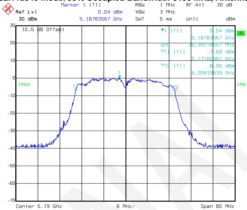
**802.11ac40 mode, 99% Occupied Bandwidth-5230 MHz, Antenna 2**
