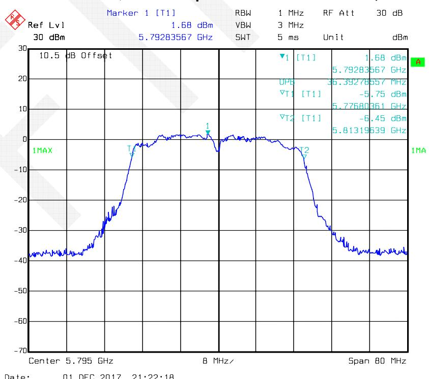
**802.11n-HT40 mode, 99% Occupied Bandwidth-5755 MHz, Antenna 2**
