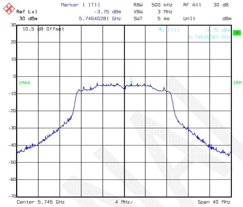
**802.11ac20 mode, Power Spectral Density-5785 MHz, Antenna 1**
