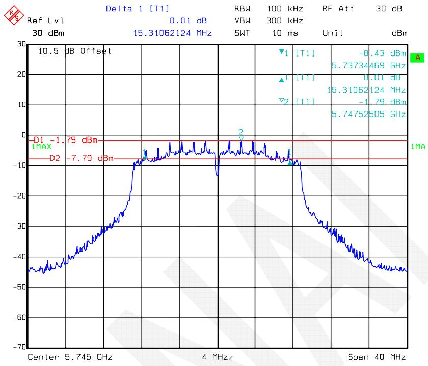
**802.11ac20 mode, 6 dB Bandwidth-5785 MHz, Antenna 1**
