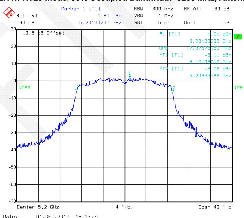
**802.11n-HT20 mode, 99% Occupied Bandwidth -5240 MHz, Antenna 1**
