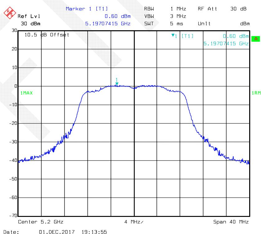
**802.11n-HT20 mode, Power Spectral Density-5240 MHz, Antenna 1**
