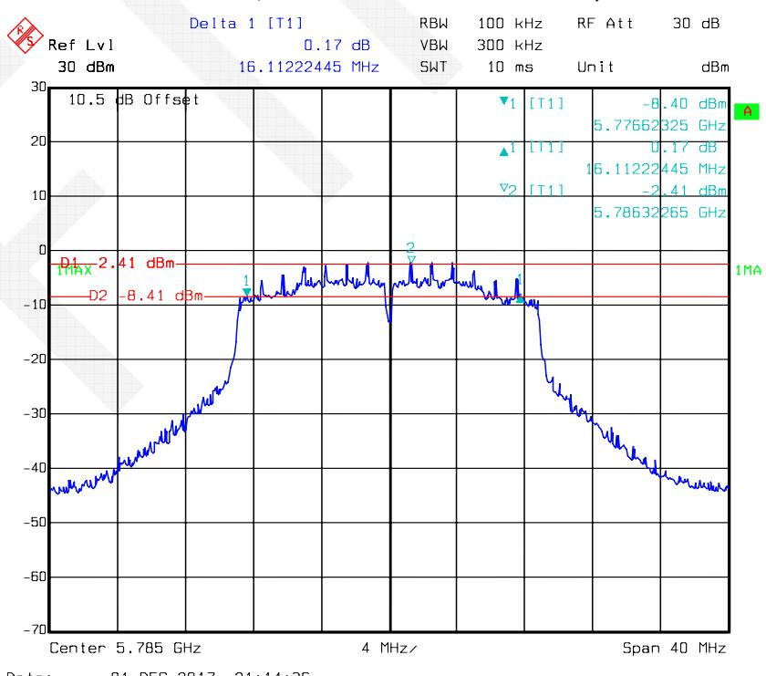
**802.11ac20 mode, 6 dB Bandwidth-5825 MHz, Antenna 1**
