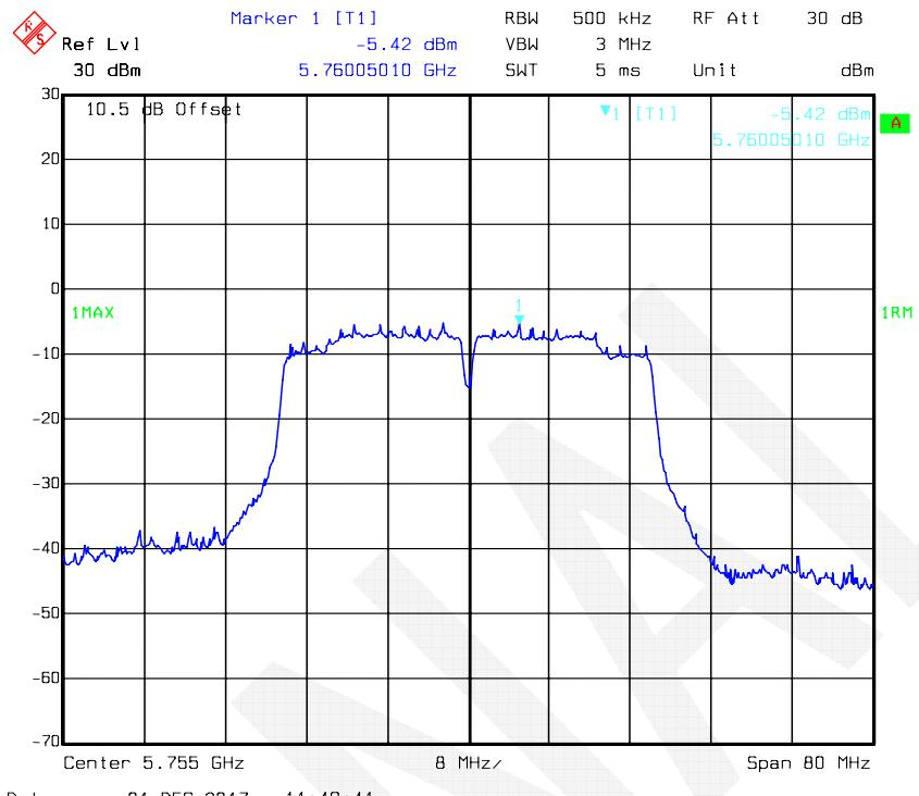
802.11n-HT40 mode, Power Spectral Density-5795 MHz, Antenna 2
