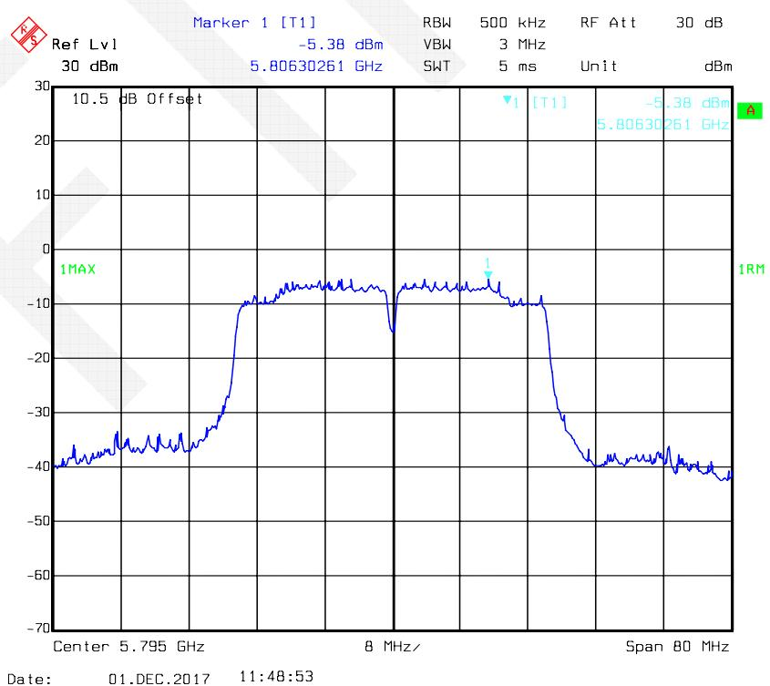
**802.11ac20 mode, Power Spectral Density-5745 MHz, Antenna 1**
