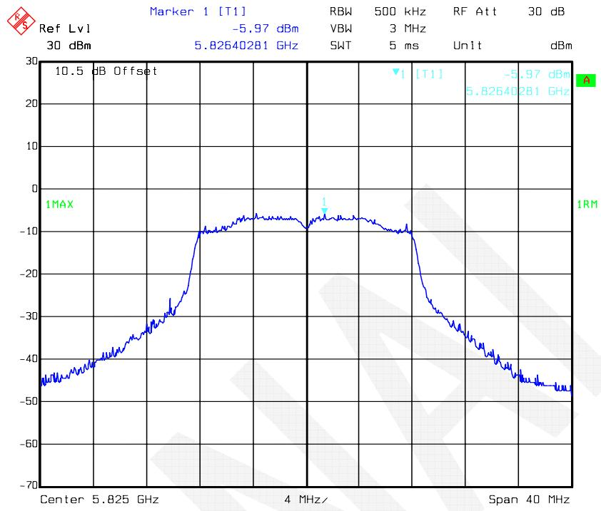
**802.11a mode, Power Spectral Density-5745 MHz, Antenna 2**
