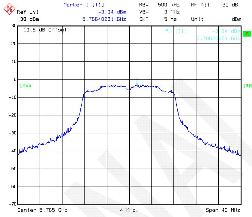
**802.11a mode, Power Spectral Density-5825 MHz, Antenna 2**
