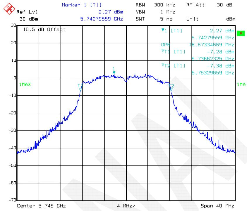
**802.11a mode, 99% Occupied Bandwidth -5785 MHz, Antenna 1**
