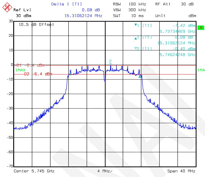
**802.11a mode, 6 dB Bandwidth-5785 MHz, Antenna 1**
