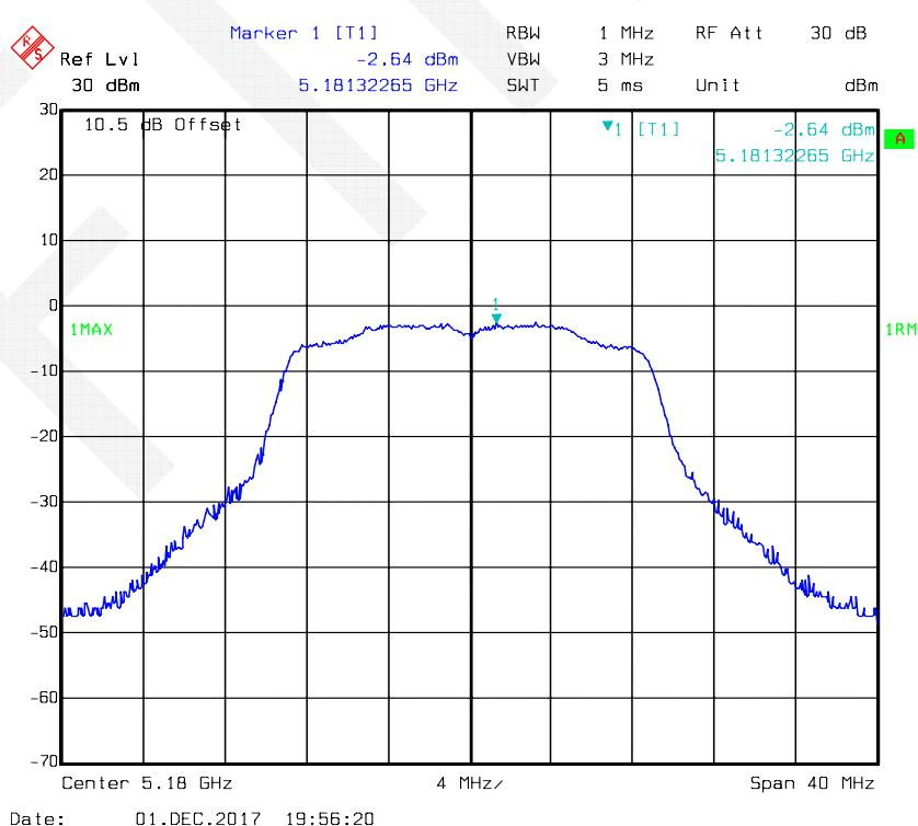
**802.11ac20 mode, Power Spectral Density-5200 MHz, Antenna 2**
