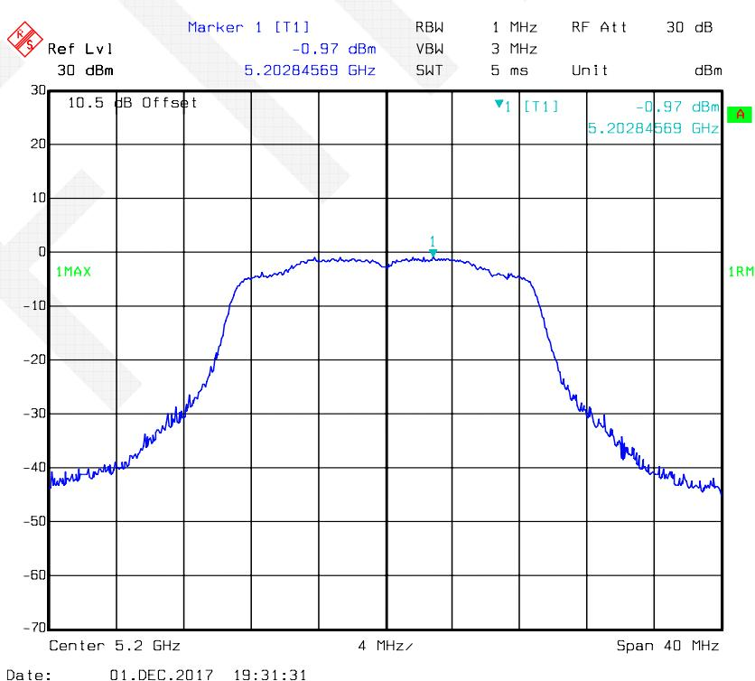
**802.11ac20 mode, Power Spectral Density-5240 MHz, Antenna 1**
