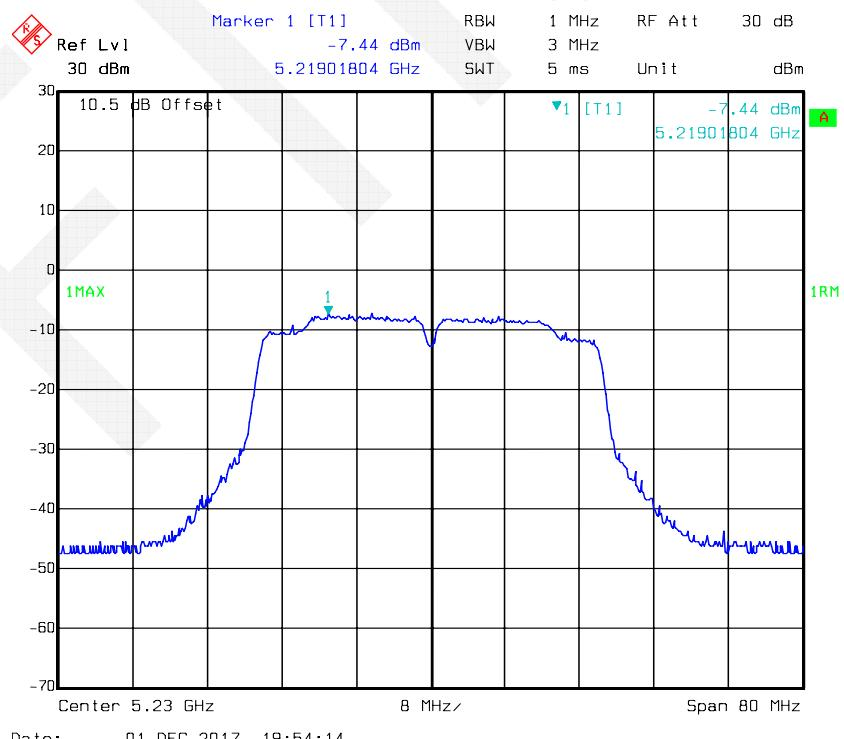
**802.11ac 80 mode, Power Spectral Density-5210 MHz, Antenna 1**
