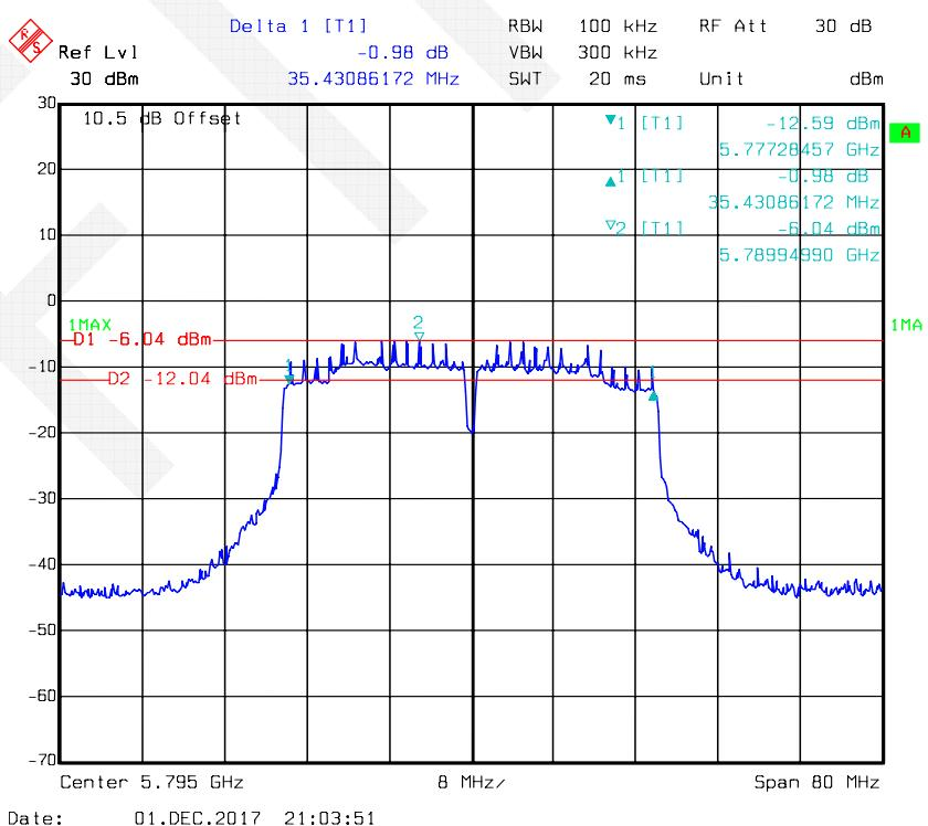
**802.11ac40 mode, 6 dB Bandwidth-5755 MHz, Antenna 2**
