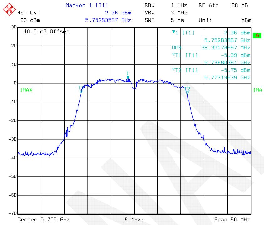
**802.11n-HT40 mode, 99% Occupied Bandwidth-5795 MHz, Antenna 1**
