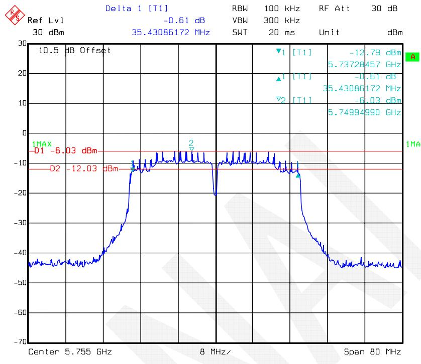
**802.11ac40 mode, 6 dB Bandwidth-5795 MHz, Antenna 2**
