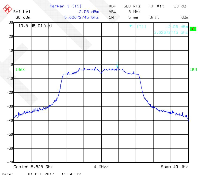
**802.11ac40 mode, Power Spectral Density-5755 MHz, Antenna 1**
