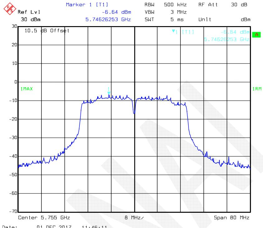
**802.11n-HT40 mode, Power Spectral Density-5795 MHz, Antenna 1**
