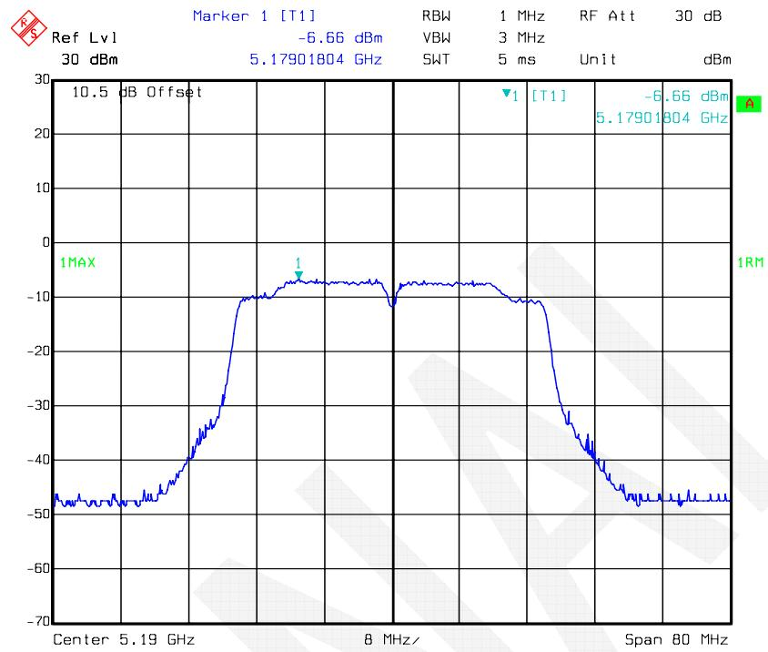
**802.11ac40 mode, Power Spectral Density-5230 MHz, Antenna 2**
