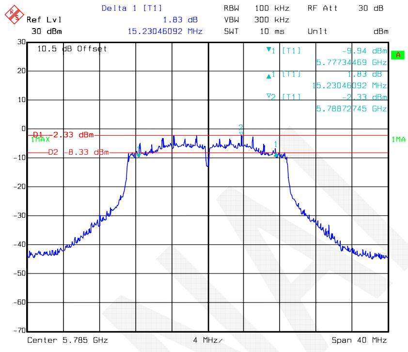
**802.11ac20 mode, 6 dB Bandwidth-5825 MHz, Antenna 2**
