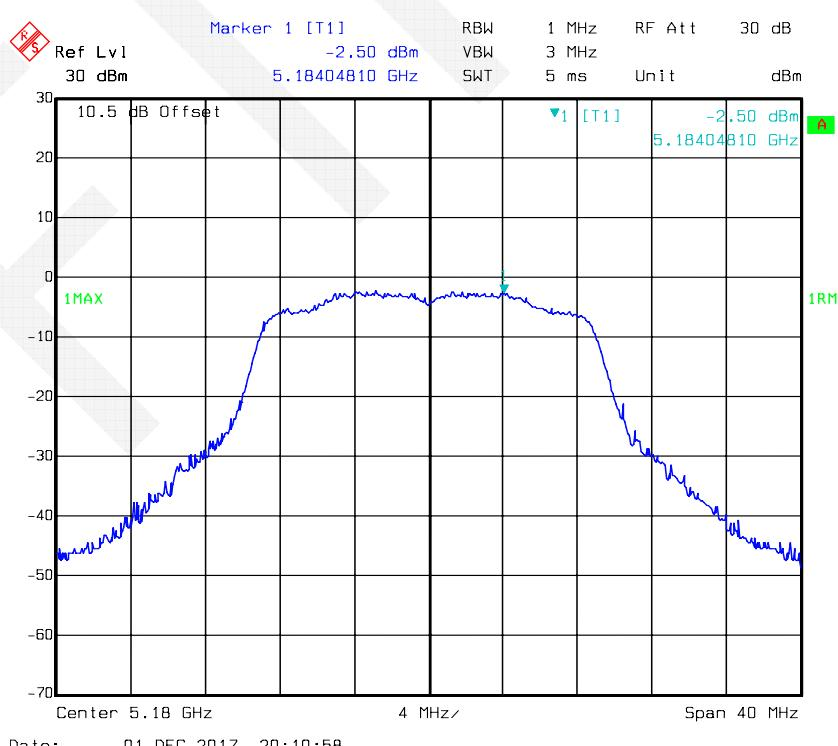
**802.11n-HT20 mode, Power Spectral Density-5200 MHz, Antenna 2**
