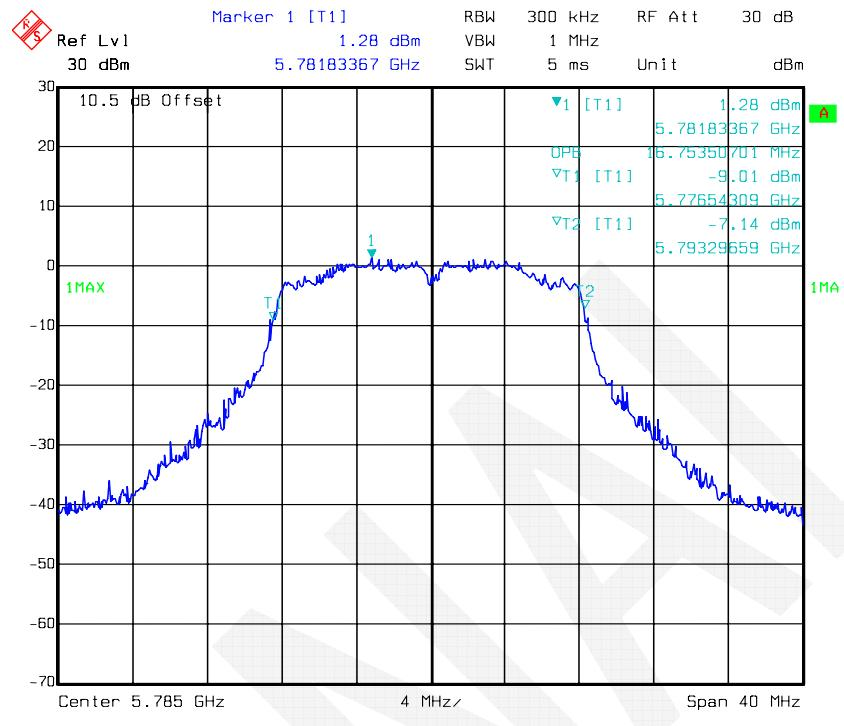
**802.11a mode, 99% Occupied Bandwidth -5825 MHz, Antenna 2**
