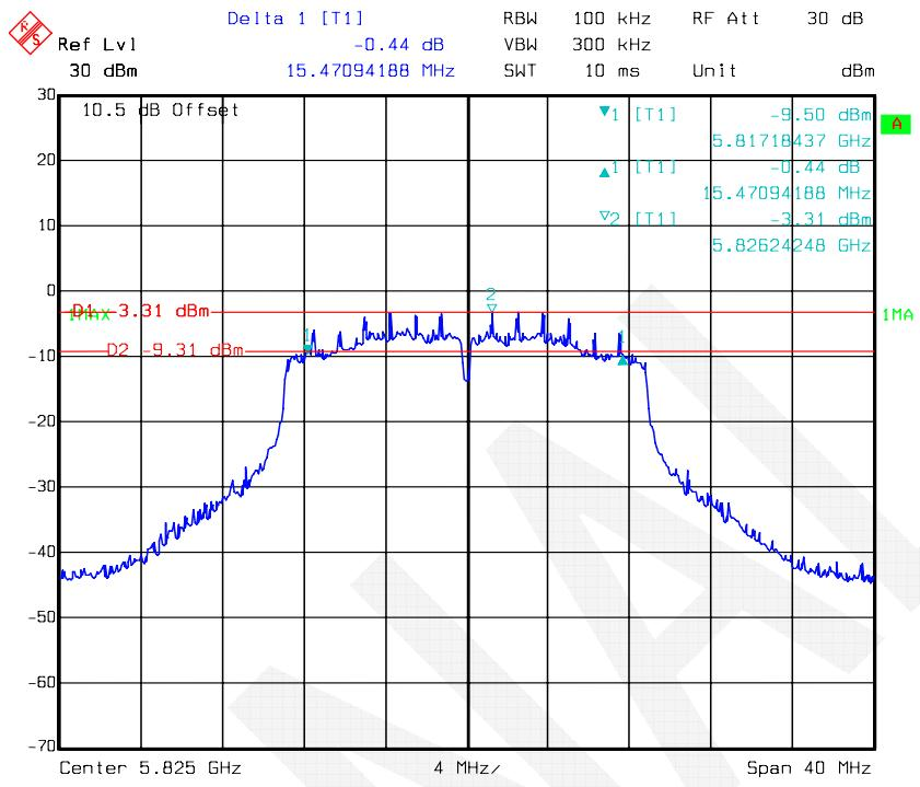
**802.11ac20 mode, 6 dB Bandwidth-5745 MHz, Antenna 2**
