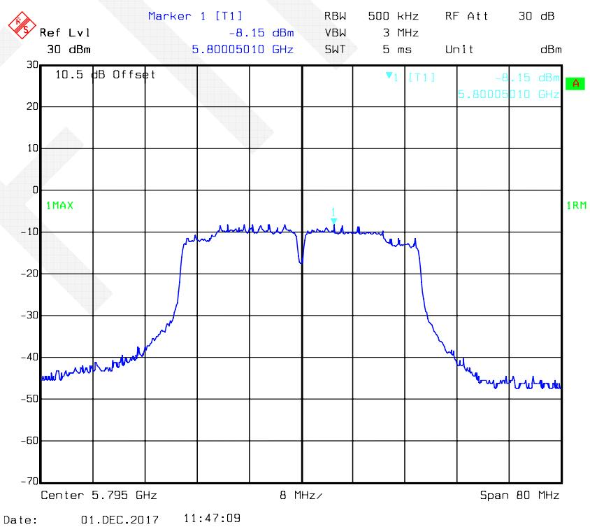
802.11n-HT40 mode, Power Spectral Density-5755 MHz, Antenna 2
