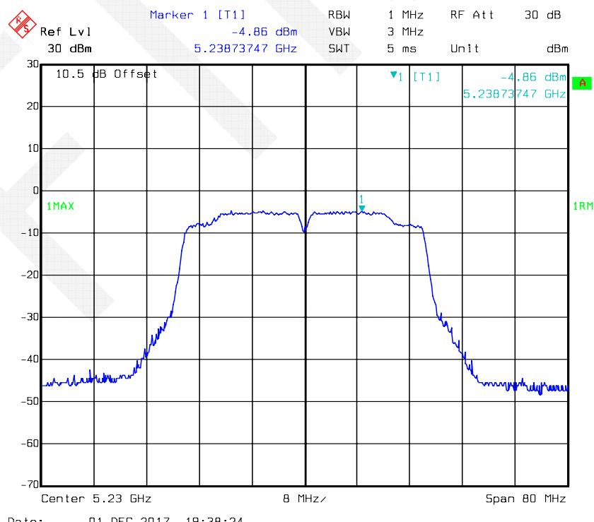
**802.11ac40 mode, Power Spectral Density-5190 MHz, Antenna 2**
