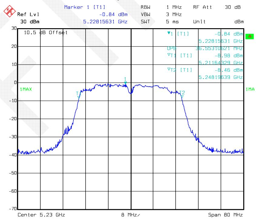
**802.11ac20 mode, 99% Occupied Bandwidth-5180 MHz, Antenna 1**
