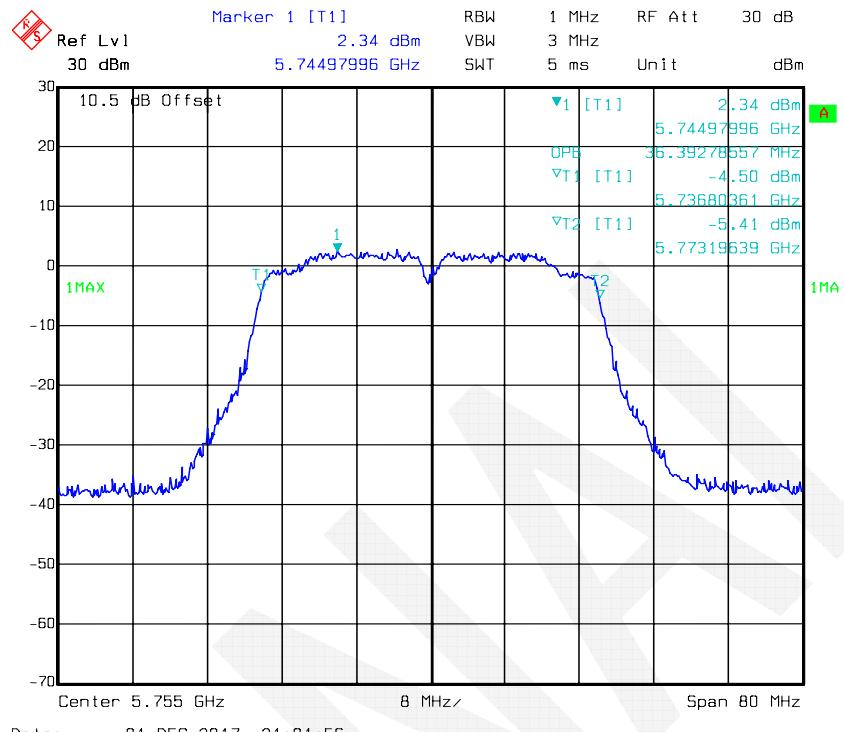
**802.11ac40 mode, 99% Occupied Bandwidth-5795 MHz, Antenna 1**
