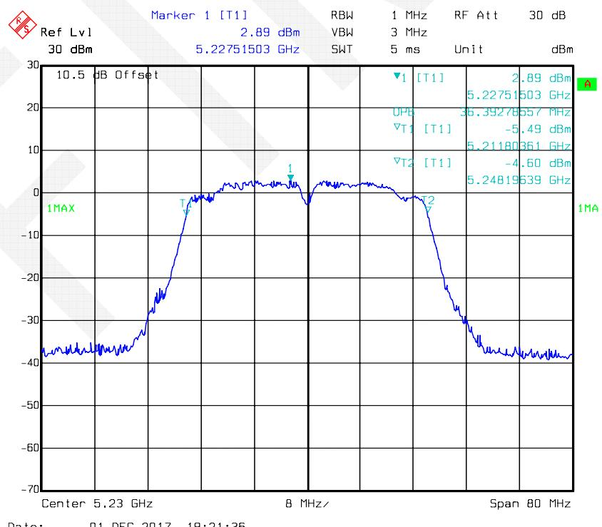
**802.11ac40 mode, 99% Occupied Bandwidth-5190 MHz, Antenna 2**
