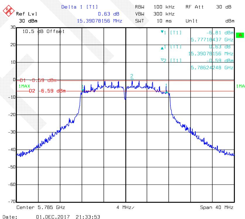
**802.11a mode, 6 dB Bandwidth-5825 MHz, Antenna 1**
