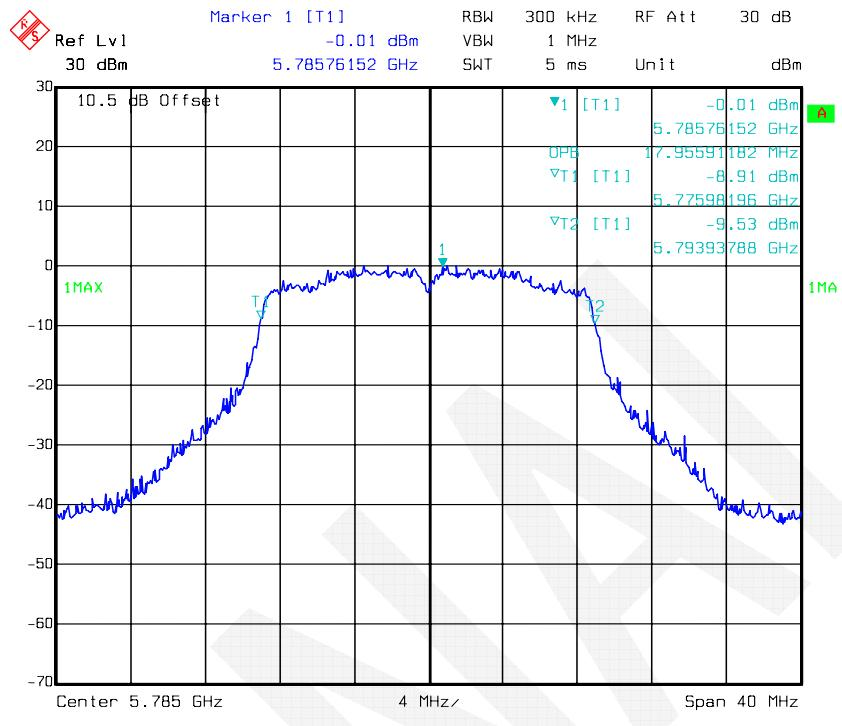
**802.11ac20 mode, 99% Occupied Bandwidth-5825 MHz, Antenna 2**
