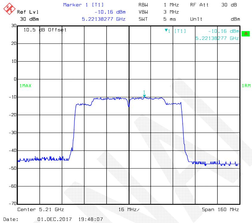
**802.11ac 80 mode, Power Spectral Density-5210 MHz, Antenna 2**
