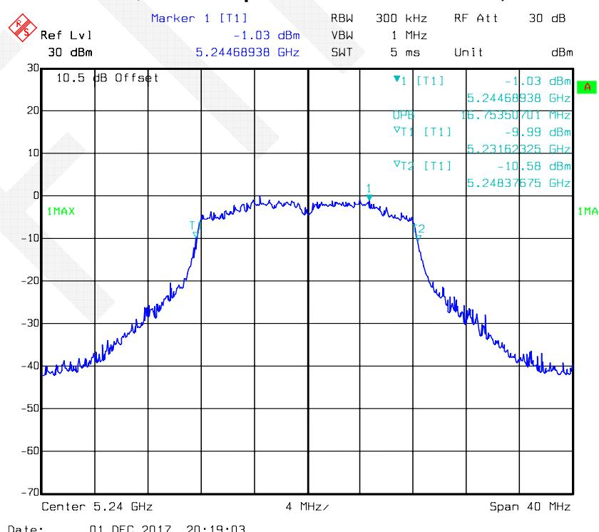
**802.11n-HT20 mode, 99% Occupied Bandwidth-5180 MHz, Antenna 1**
