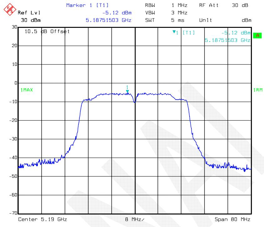
**802.11n-HT40 mode, Power Spectral Density-5230 MHz, Antenna 1**
