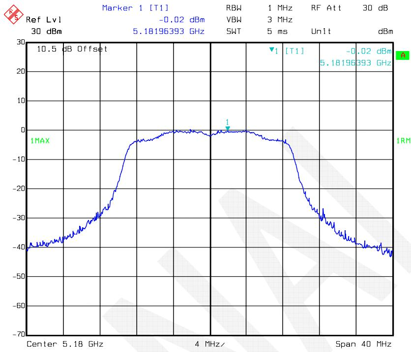
**802.11ac20 mode, Power Spectral Density-5200 MHz, Antenna 1**
