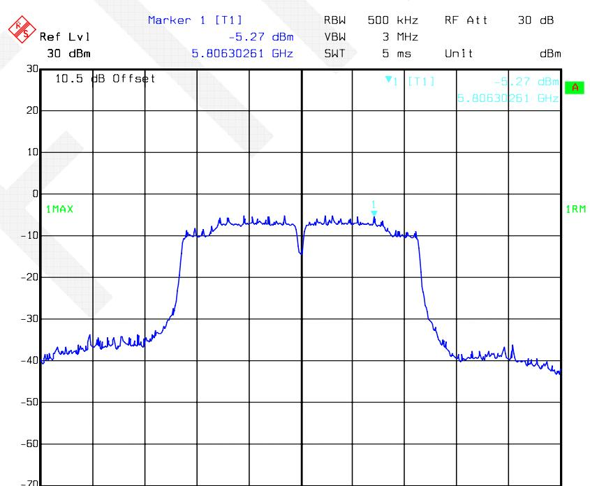
**802.11ac80 mode, Power Spectral Density-5775 MHz, Antenna 1**
