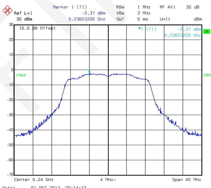
**802.11n-HT40 mode, Power Spectral Density-5190 MHz, Antenna 1**
