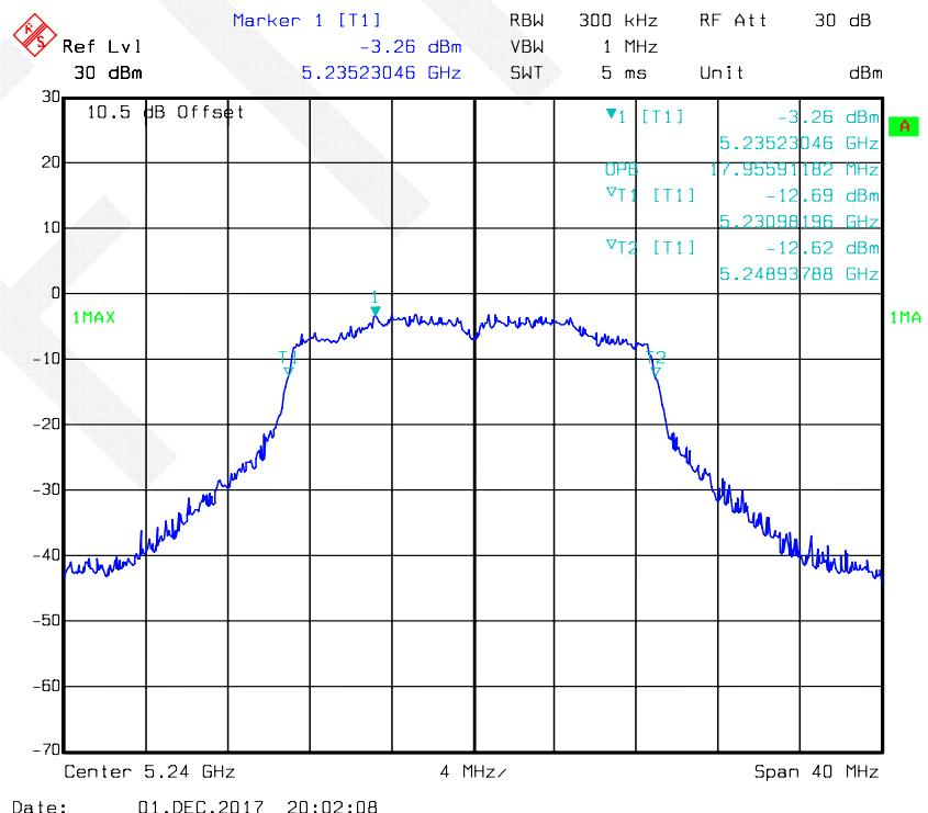
**802.11ac40 mode, 99% Occupied Bandwidth-5190 MHz, Antenna 1**
