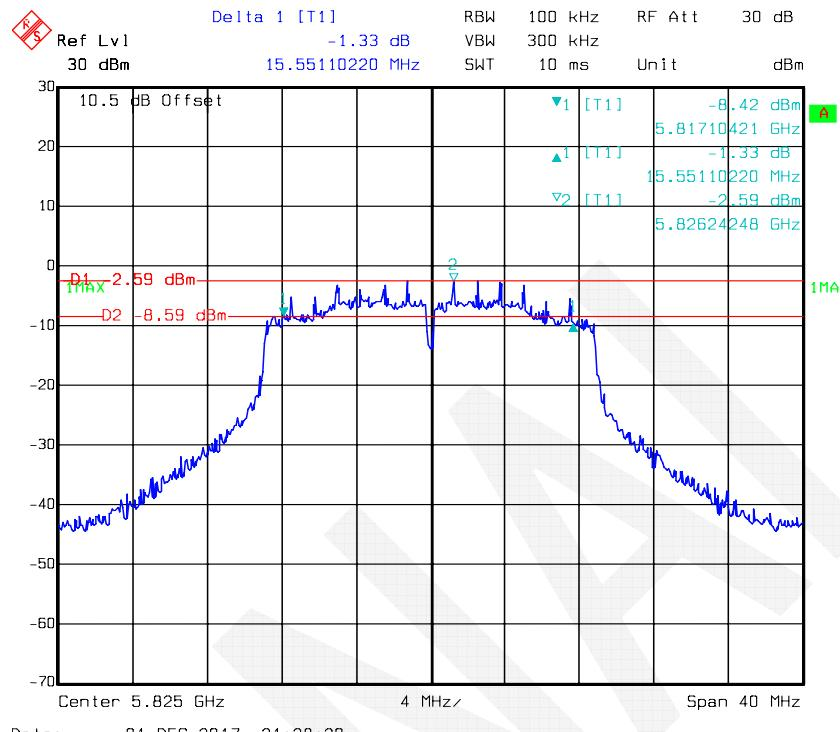
**802.11n-HT20 mode, 6 dB Bandwidth-5745 MHz, Antenna 2**
