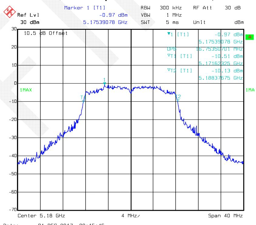
**802.11a mode, 99% Occupied Bandwidth -5200 MHz, Antenna 2**
