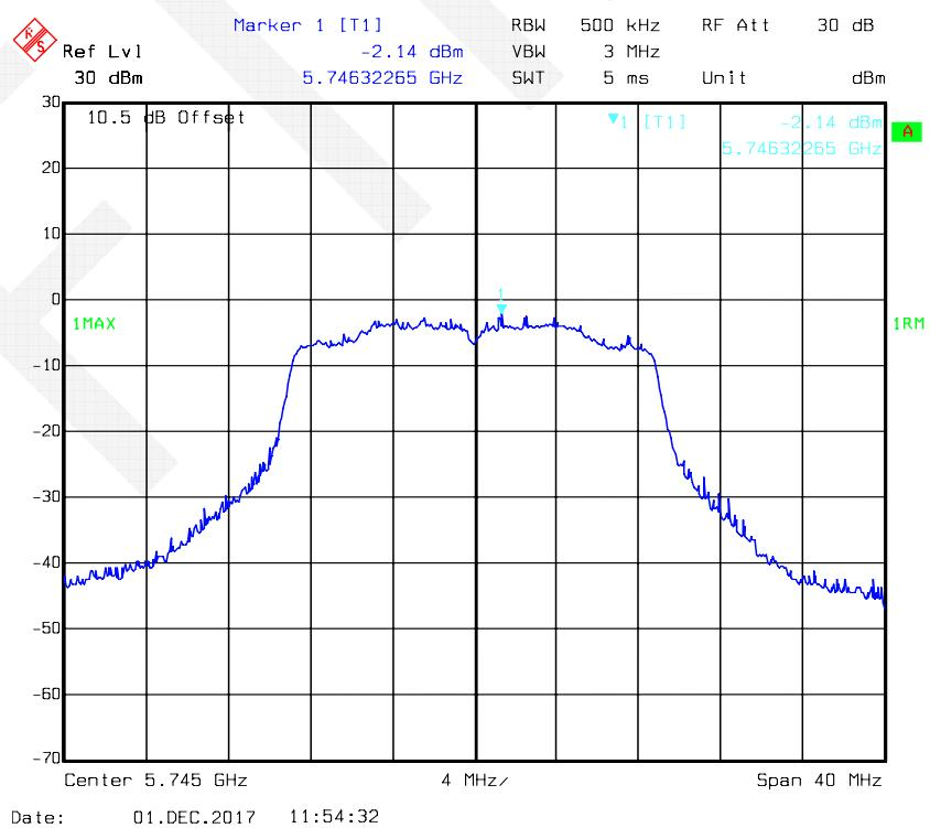
**802.11ac20 mode, Power Spectral Density-5785 MHz, Antenna 2**
