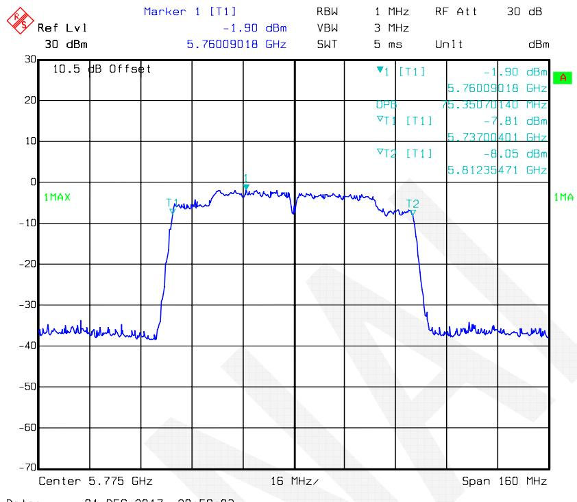
**802.11ac80 mode, 99% Occupied Bandwidth-5775 MHz, Antenna 2**
