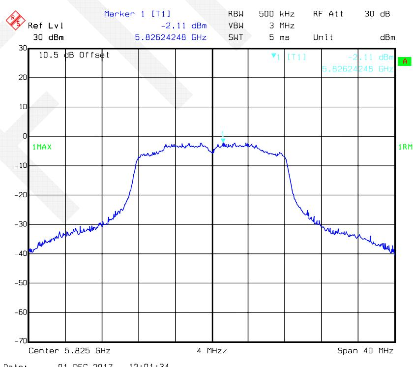
**802.11n-HT20 mode, Power Spectral Density-5745 MHz, Antenna 1**
