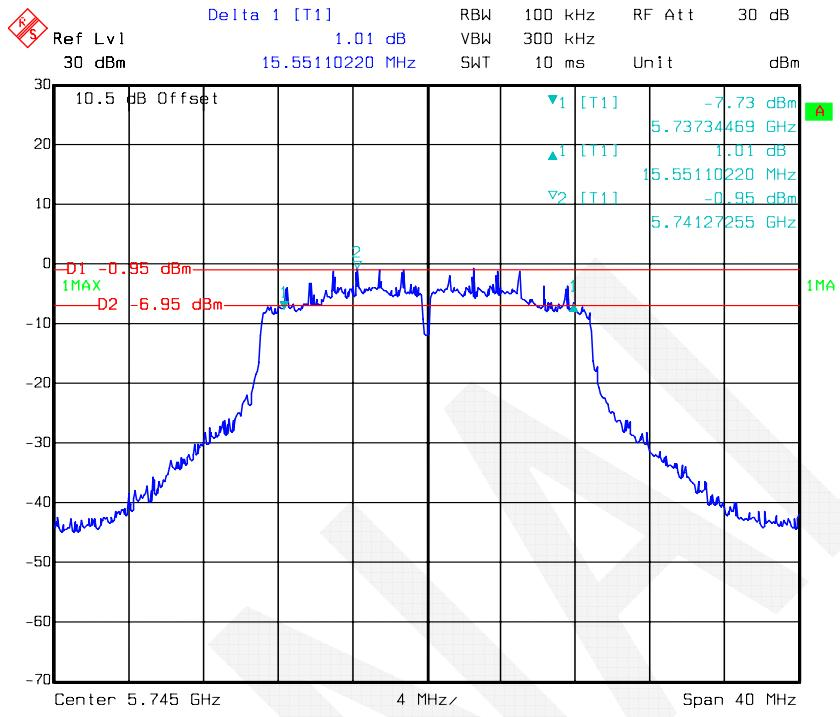
**802.11n-HT20 mode, 6 dB Bandwidth-5785 MHz, Antenna 1**
