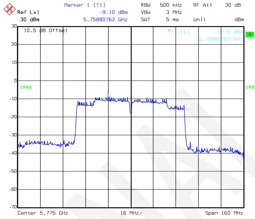
**802.11ac80 mode, Power Spectral Density-5775 MHz, Antenna 2**
