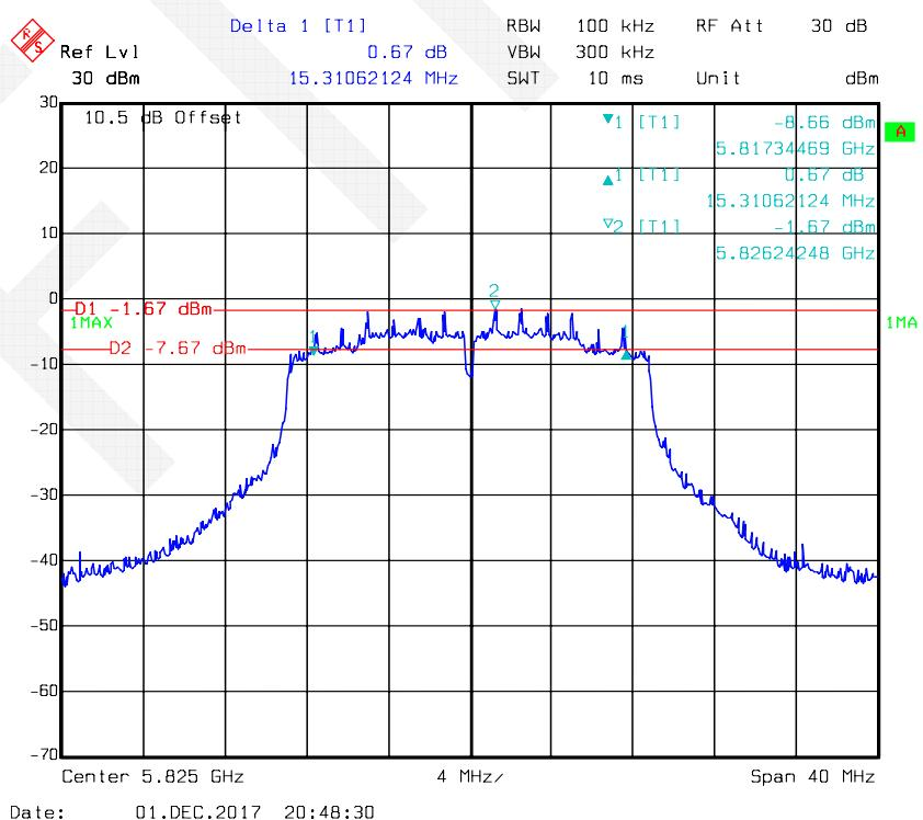
**802.11ac40 mode, 6 dB Bandwidth-5755 MHz, Antenna 1**
