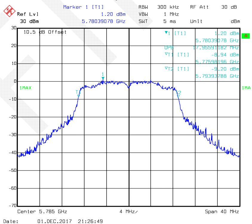
**802.11n-HT20 mode, 99% Occupied Bandwidth-5825 MHz, Antenna 1**
