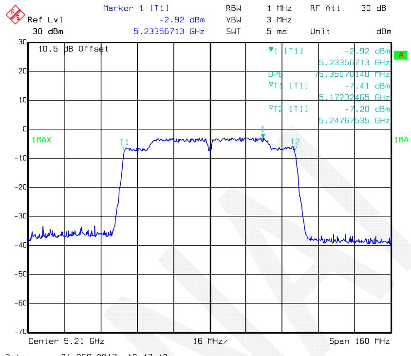
**802.11ac80 mode, 99% Occupied Bandwidth-5210 MHz, Antenna 2**
