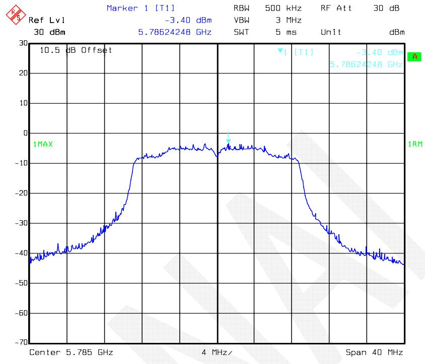
802.11n-HT20 mode Power Spectral Density-5825 MHz Antenna 2
