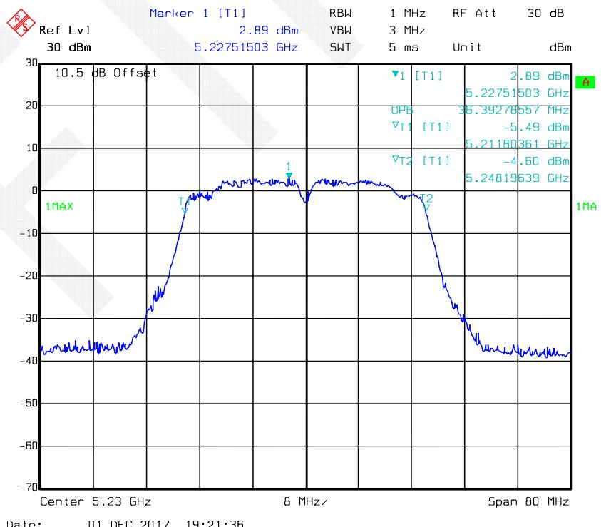
**802.11n-HT40 mode, 99% Occupied Bandwidth-5190 MHz, Antenna 2**
