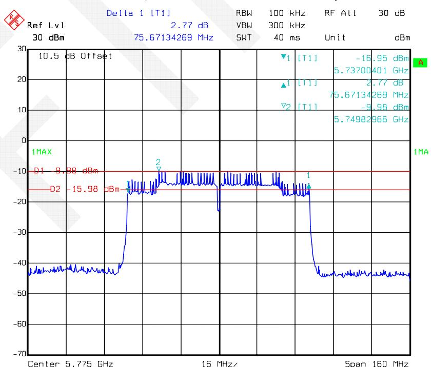
**802.11a mode, 99% Occupied Bandwidth-5745 MHz, Antenna 1**
