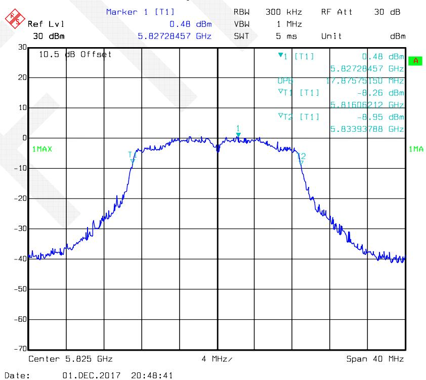
**802.11ac40 mode, 99% Occupied Bandwidth-5755 MHz, Antenna 1**
