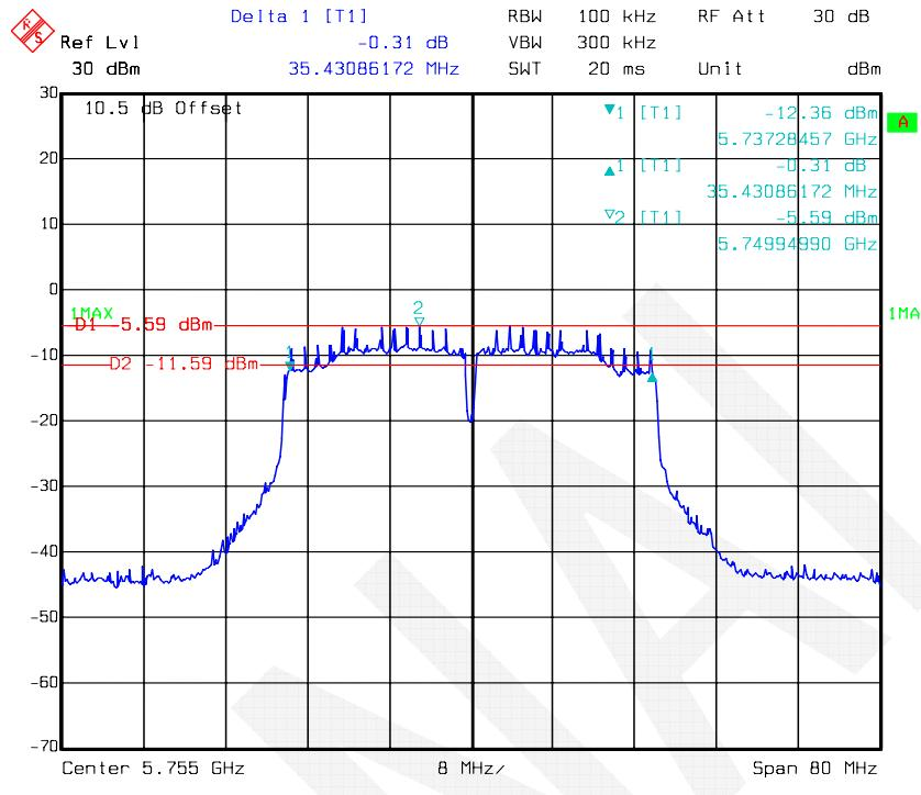
**802.11n-HT40 mode, 6 dB Bandwidth-5795 MHz, Antenna 1**
