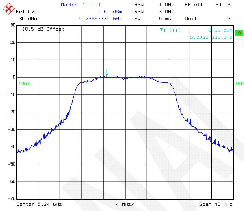
**802.11n-HT20 mode, Power Spectral Density-5180 MHz, Antenna 2**
