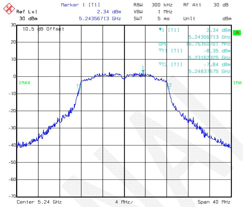
**802.11a mode, 99% Occupied Bandwidth-5180 MHz, Antenna 2**
