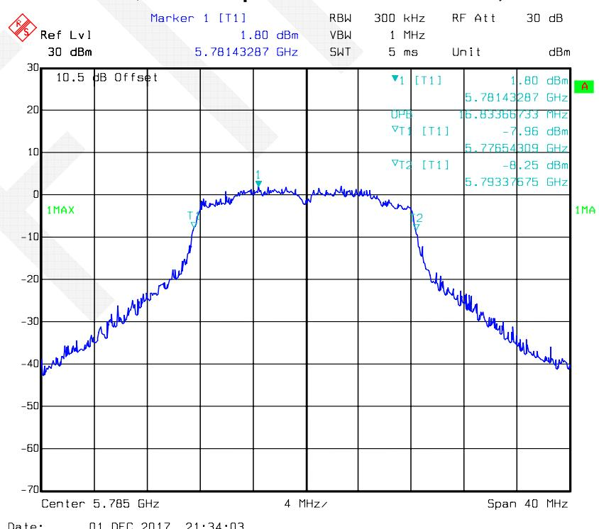
**802.11a mode, 99% Occupied Bandwidth -5825 MHz, Antenna 1**
