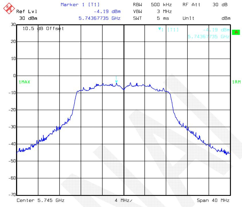
**802.11n-HT20 mode, Power Spectral Density-5785 MHz, Antenna 1**
