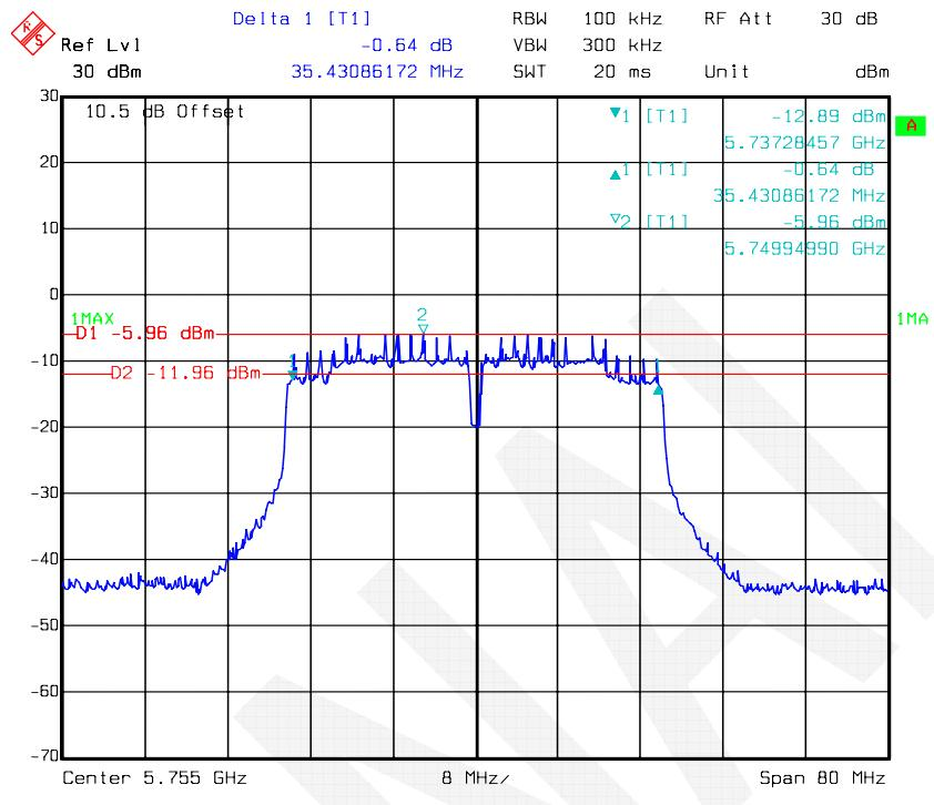
**802.11n-HT40 mode, 6 dB Bandwidth-5795 MHz, Antenna 2**
