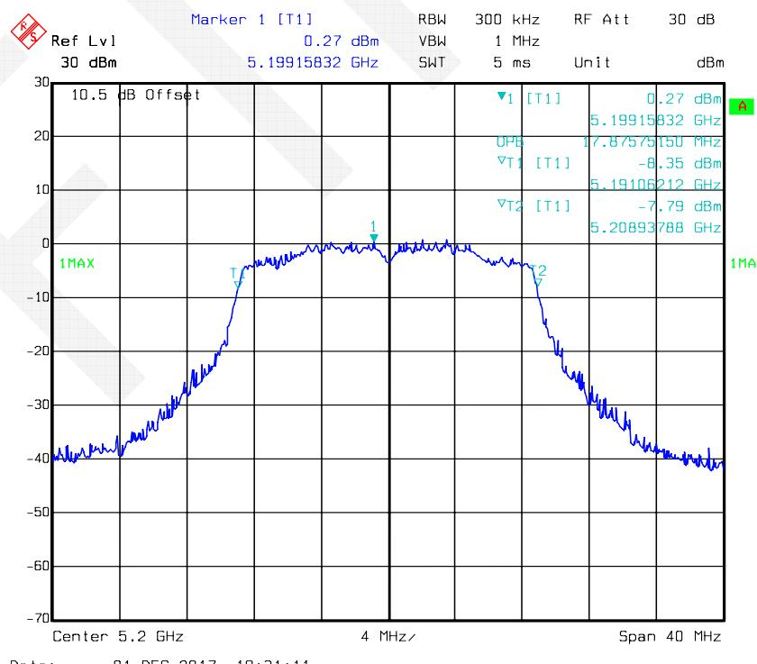
**802.11ac20 mode, 99% Occupied Bandwidth-5240 MHz, Antenna 1**
