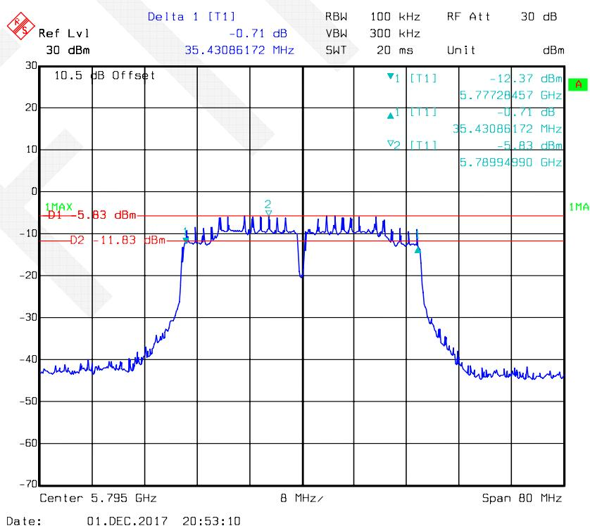
**802.11ac80 mode, 6 dB Bandwidth-5775 MHz, Antenna 1**
