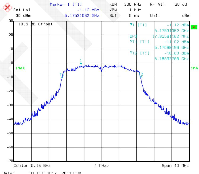
**802.11n-HT20 mode, 99% Occupied Bandwidth -5200 MHz, Antenna 2**
