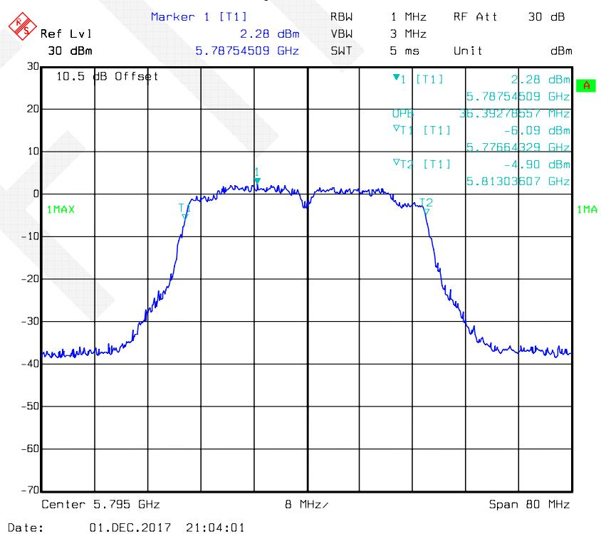
**802.11ac40 mode, 99% Occupied Bandwidth-5755 MHz, Antenna 2**
