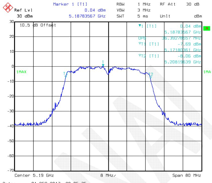
**802.11n-HT40 mode, 99% Occupied Bandwidth-5230 MHz, Antenna 2**
