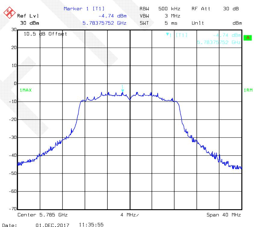
**802.11ac20 mode, Power Spectral Density-5825 MHz, Antenna 1**
