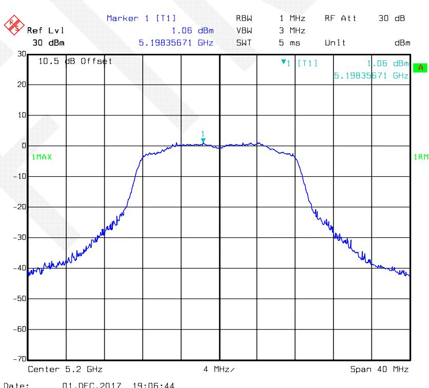
**802.11a mode, Power Spectral Density-5240 MHz, Antenna 1**
