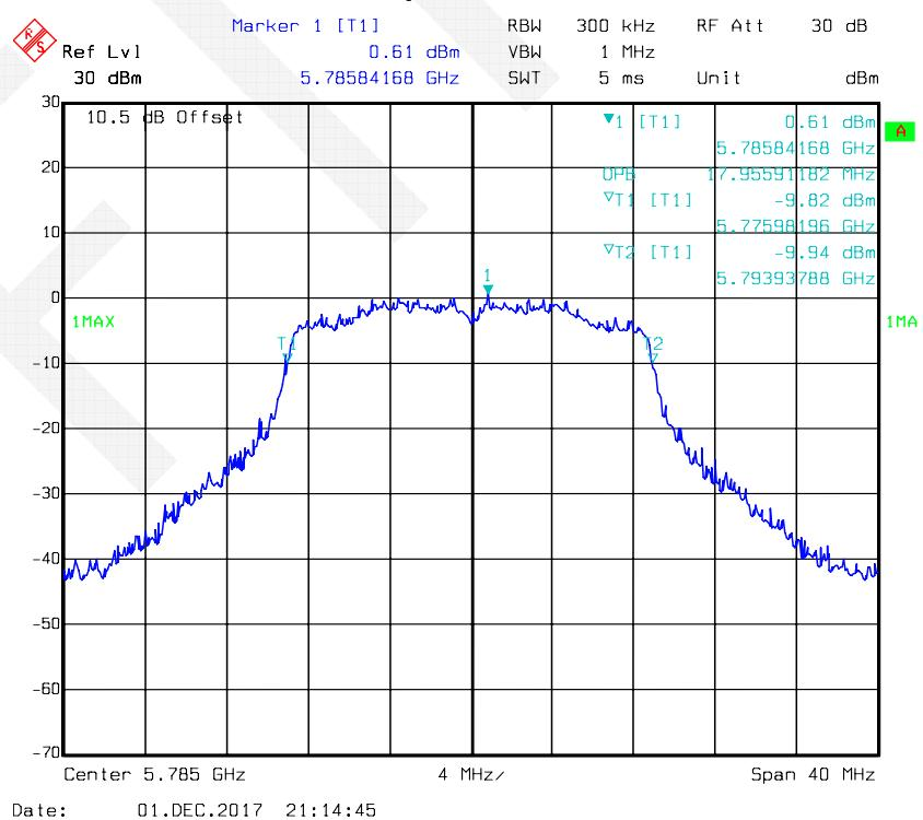
**802.11ac20 mode, 99% Occupied Bandwidth-5825 MHz, Antenna 1**
