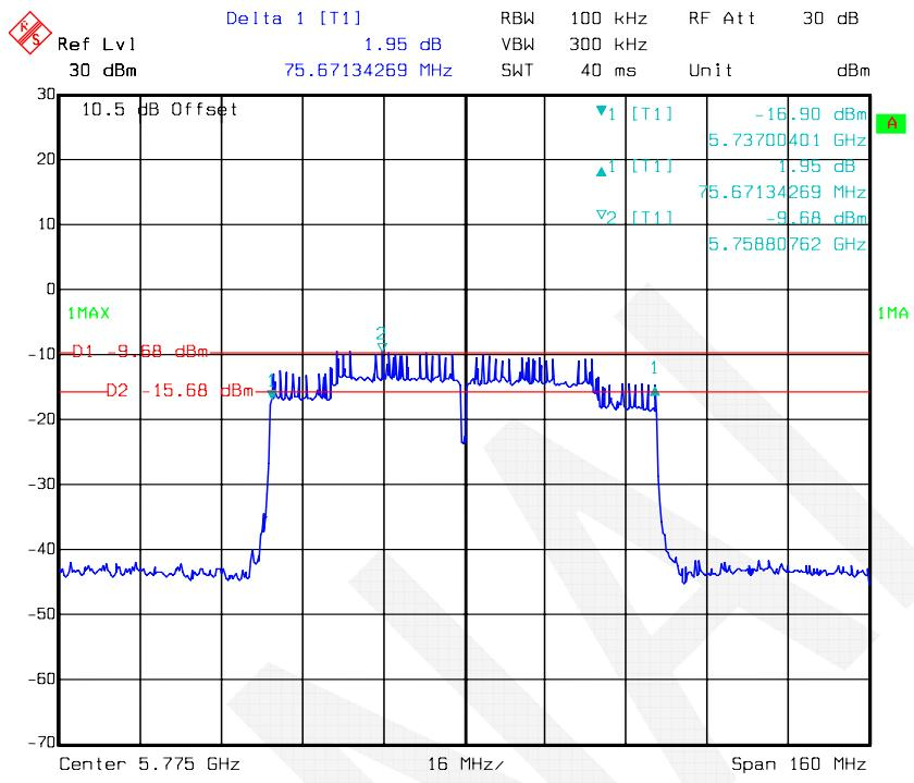
**802.11ac80 mode, 6 dB Bandwidth-5775 MHz, Antenna 2**
