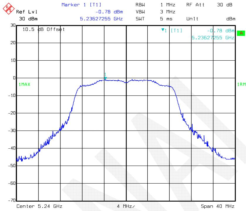
**802.11ac20 mode, Power Spectral Density-5180 MHz, Antenna 2**
