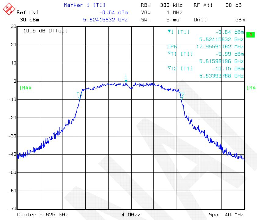
**802.11n-HT20 mode, 99% Occupied Bandwidth-5745 MHz, Antenna 2**
