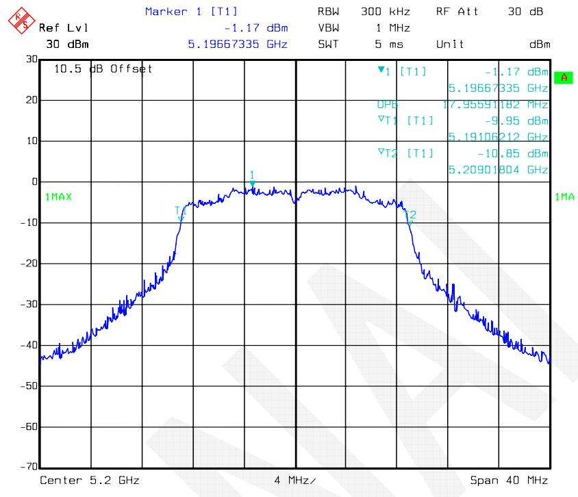
**802.11n-HT20 mode, 99% Occupied Bandwidth -5240 MHz, Antenna 2**
