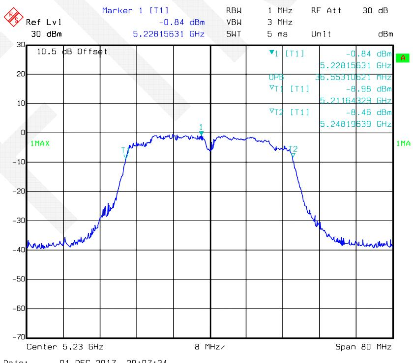
**802.11ac80 mode, 99% Occupied Bandwidth-5210 MHz, Antenna 1**
