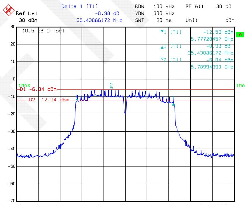
**802.11n-HT40 mode, 6 dB Bandwidth-5755 MHz, Antenna 2**
