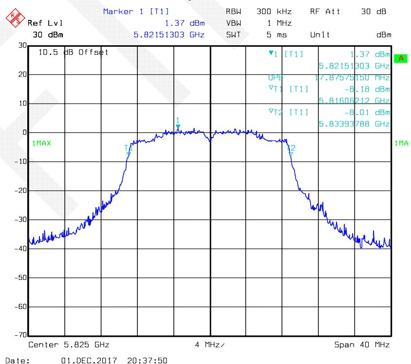
**802.11n-HT40 mode, 99% Occupied Bandwidth-5755 MHz, Antenna 1**
