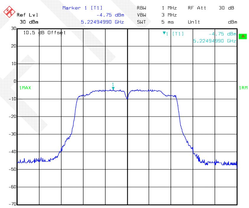
**802.11n-HT40 mode, Power Spectral Density-5190 MHz, Antenna 2**
