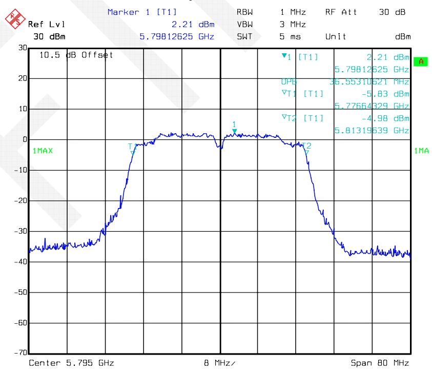
**802.11ac80 mode, 99% Occupied Bandwidth-5775 MHz, Antenna 1**
