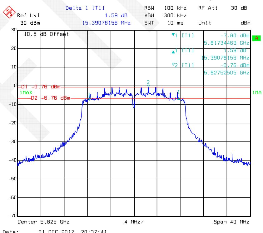
**802.11n-HT40 mode, 6 dB Bandwidth-5755 MHz, Antenna 1**
