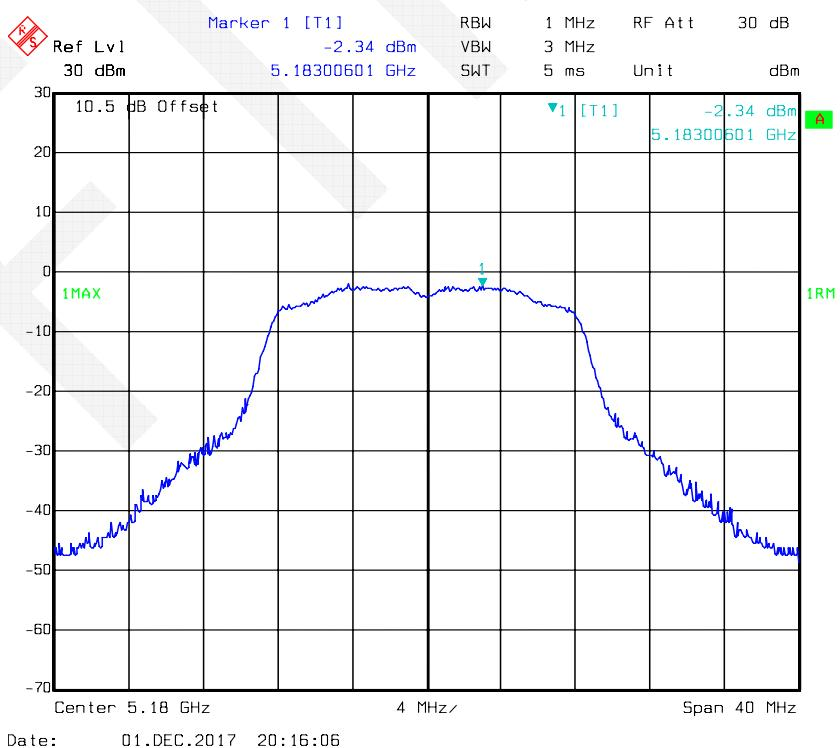
**802.11a mode, Power Spectral Density-5200 MHz, Antenna 2**
