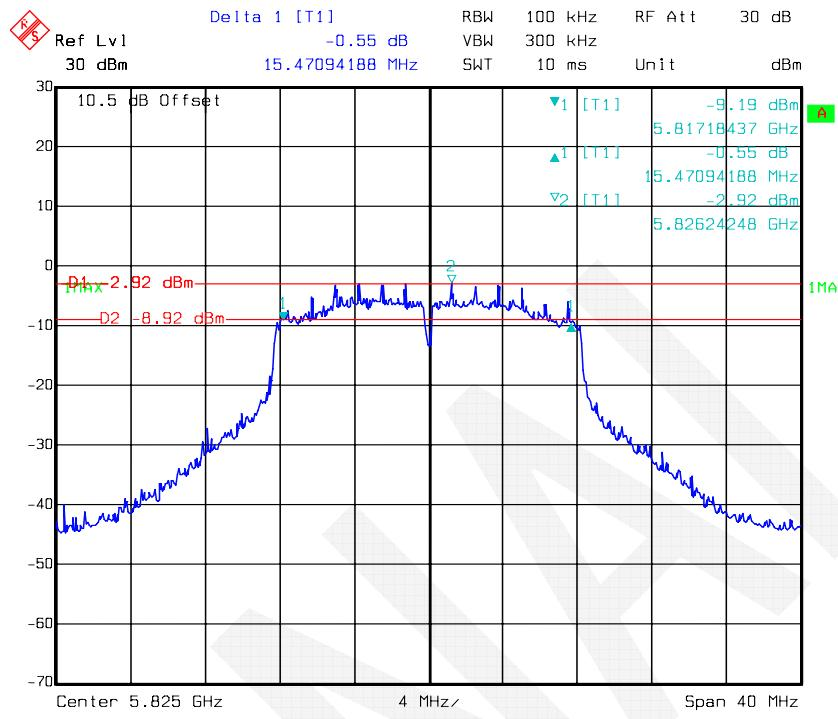
**802.11a mode, 6 dB Bandwidth-5745 MHz, Antenna 2**
