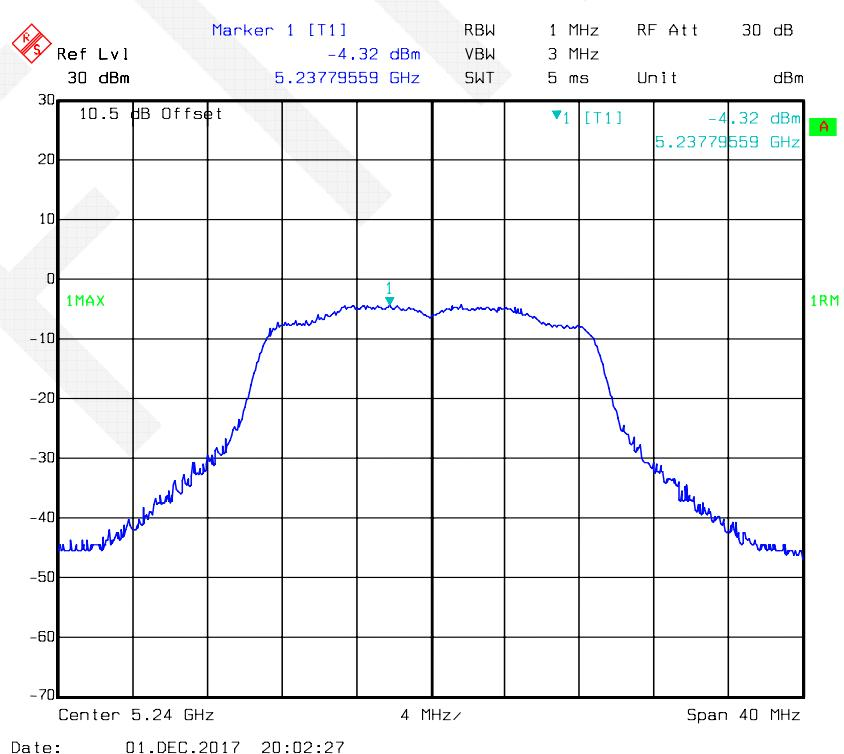
**802.11ac40 mode, Power Spectral Density-5190 MHz, Antenna 1**
