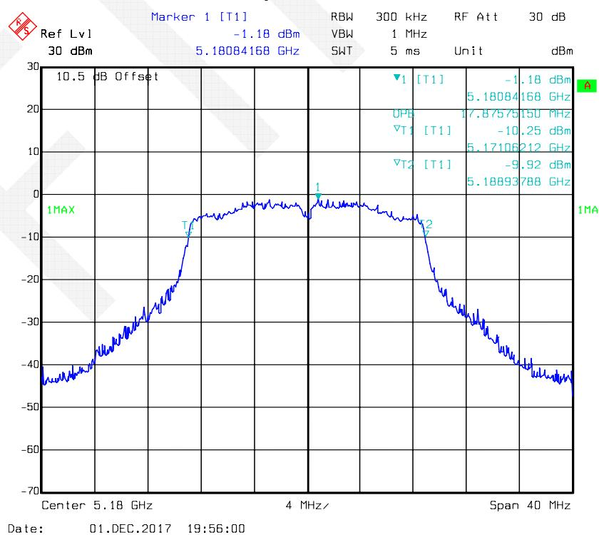
**802.11ac20 mode, 99% Occupied Bandwidth-5200 MHz, Antenna 2**
