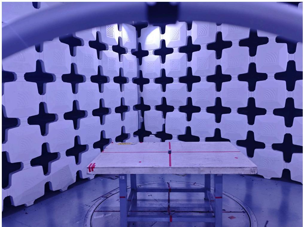
**Radiated Emissions Test Photos****30 MHz to 1000 MHz**
