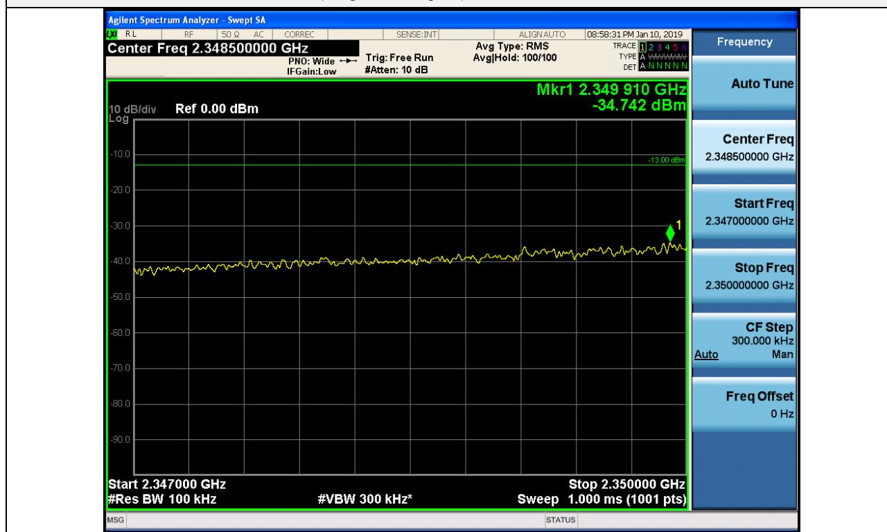
+3 dB above Out-of-band (single test signal) / BRS/EBS / Downlink / LTE 10 MHz (TDD) / Upper
