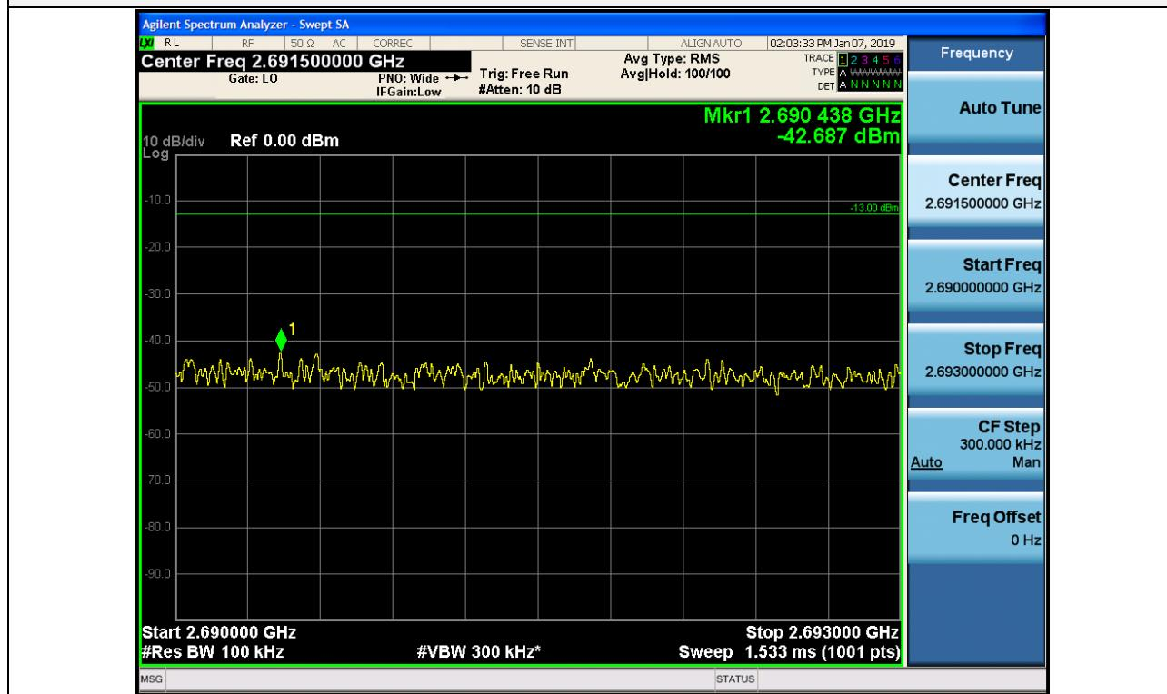
+3 dB above Out-of-band (two adjacent test signals) / BRS/EBS / Downlink / LTE 10 MHz (TDD) / Lower
