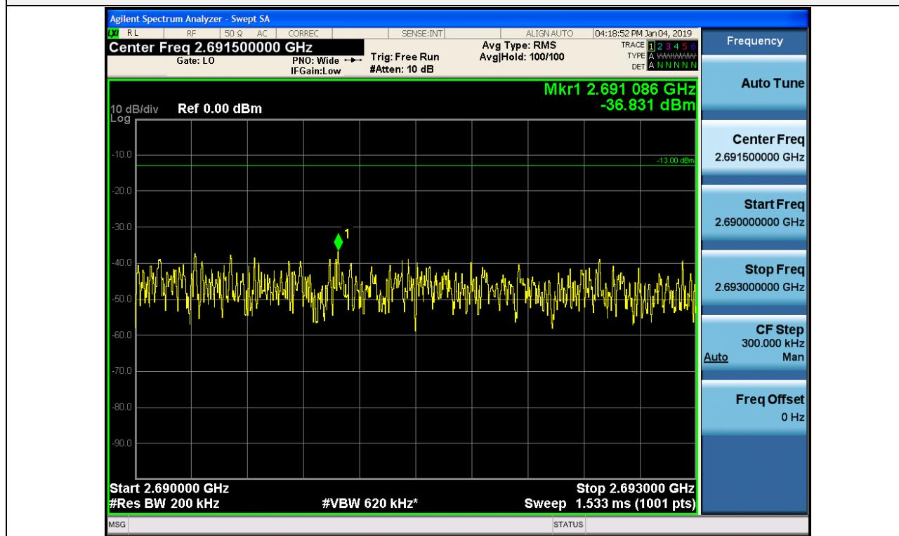
+3 dB above Out-of-band (two adjacent test signals) / BRS/EBS / Downlink / LTE 20 MHz (TDD) / Lower
