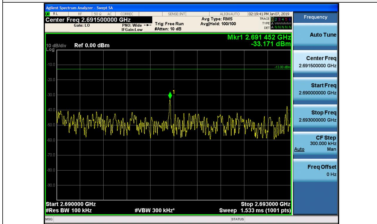
+3 dB above Out-of-band (single test signal) / BRS/EBS / Downlink / LTE 10 MHz (TDD) / Lower
