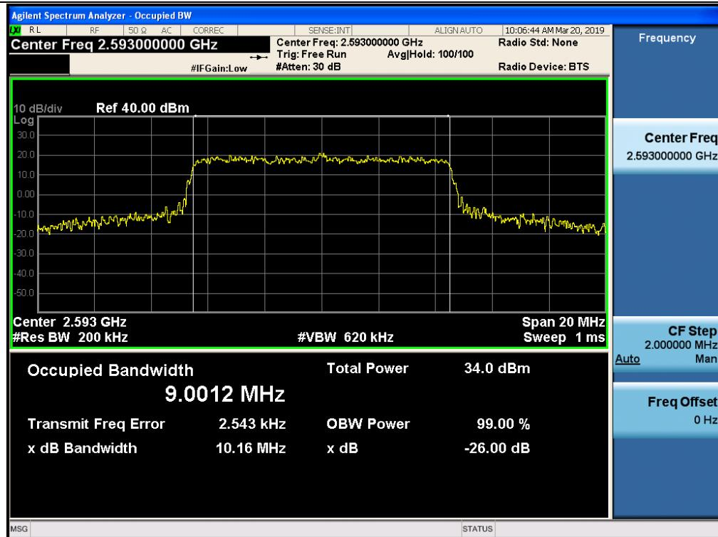
3 dB above the AGC threshold output / BRS/EBS / Downlink / LTE 20 MHz (TDD)
