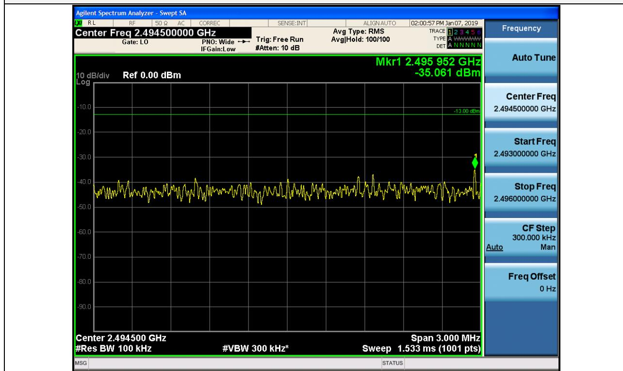
+3 dB above Out-of-band (two adjacent test signals) / BRS/EBS / Downlink / LTE 20 MHz (TDD) / Upper
