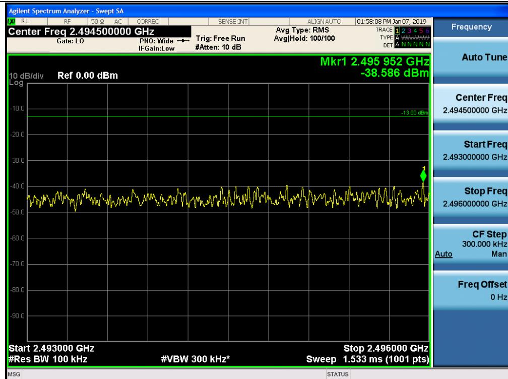
Out-of-band (two adjacent test signals) / BRS/EBS / Downlink / LTE 20 MHz (TDD) / Upper
