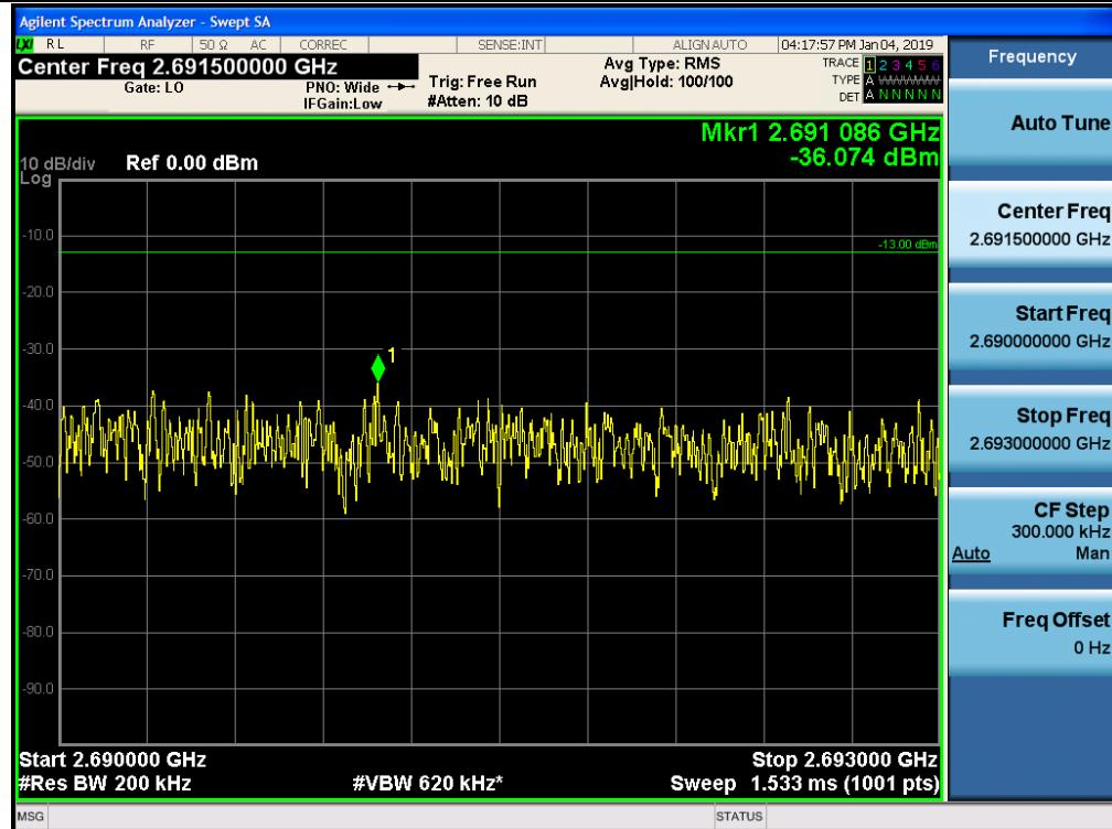
Out-of-band (two adjacent test signals) / BRS/EBS / Downlink / LTE 20 MHz (TDD) / Lower
