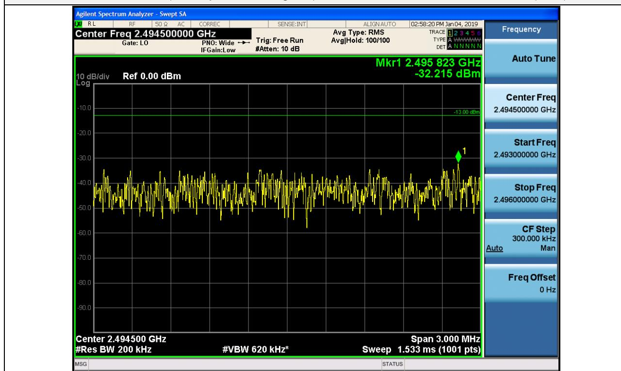
Out-of-band (single test signal) / WCS / Downlink / LTE 5 MHz / Upper
