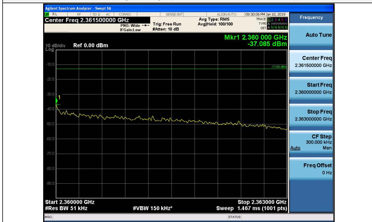
Out-of-band (single test signal) / WCS / Downlink / LTE 5 MHz / Lower
