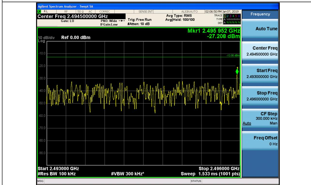
+3 dB above Out-of-band (single test signal) / BRS/EBS / Downlink / LTE 20 MHz (TDD) / Upper
