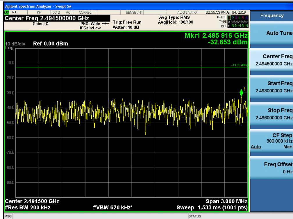
+3 dB above Out-of-band (two adjacent test signals) / WCS / Downlink / LTE 5 MHz / Upper
