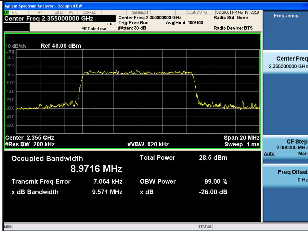
3 dB above the AGC threshold output / BRS/EBS / Downlink / LTE 10 MHz (TDD)
