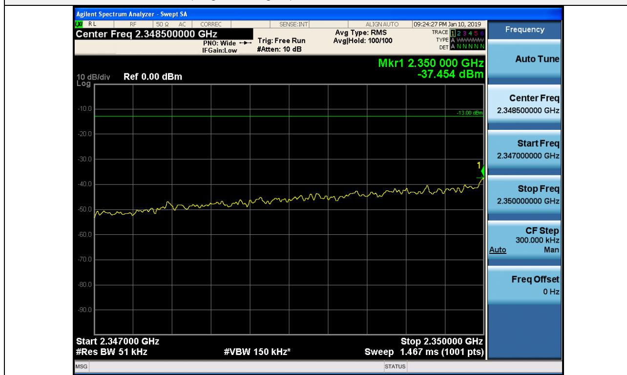
Out-of-band (single test signal) / WCS / Downlink / LTE 10 MHz / Upper
