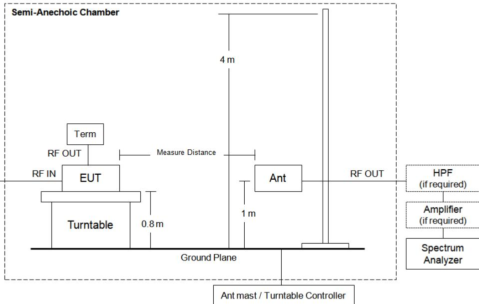
\* EUT position is adopted by placement of floor-standing refer to section 5.5.2.3.2 of ANSI C63.26-2015
