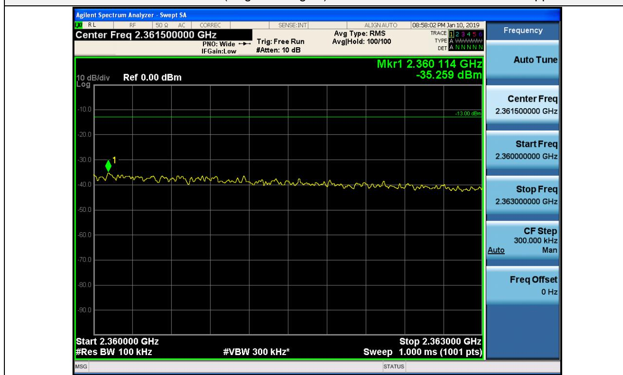
+3 dB above Out-of-band (single test signal) / WCS / Downlink / LTE 10 MHz / Lower
