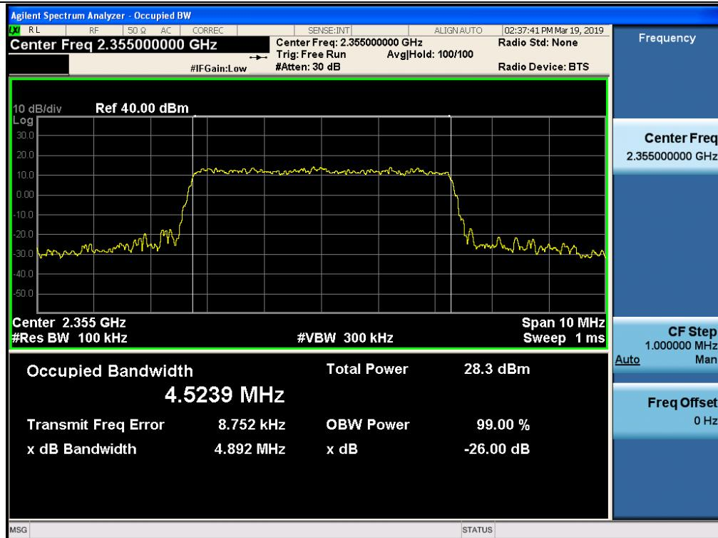
3 dB above the AGC threshold output / WCS / Downlink / LTE 10 MHz
