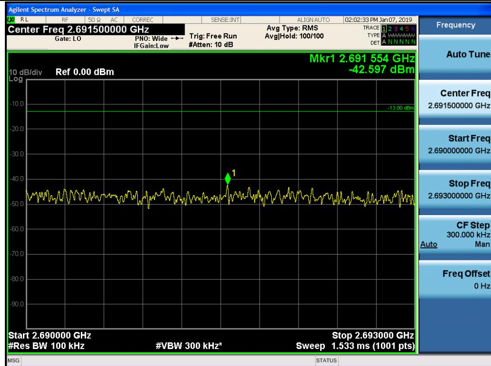
Out-of-band (two adjacent test signals) / BRS/EBS / Downlink / LTE 10 MHz (TDD) / Lower
