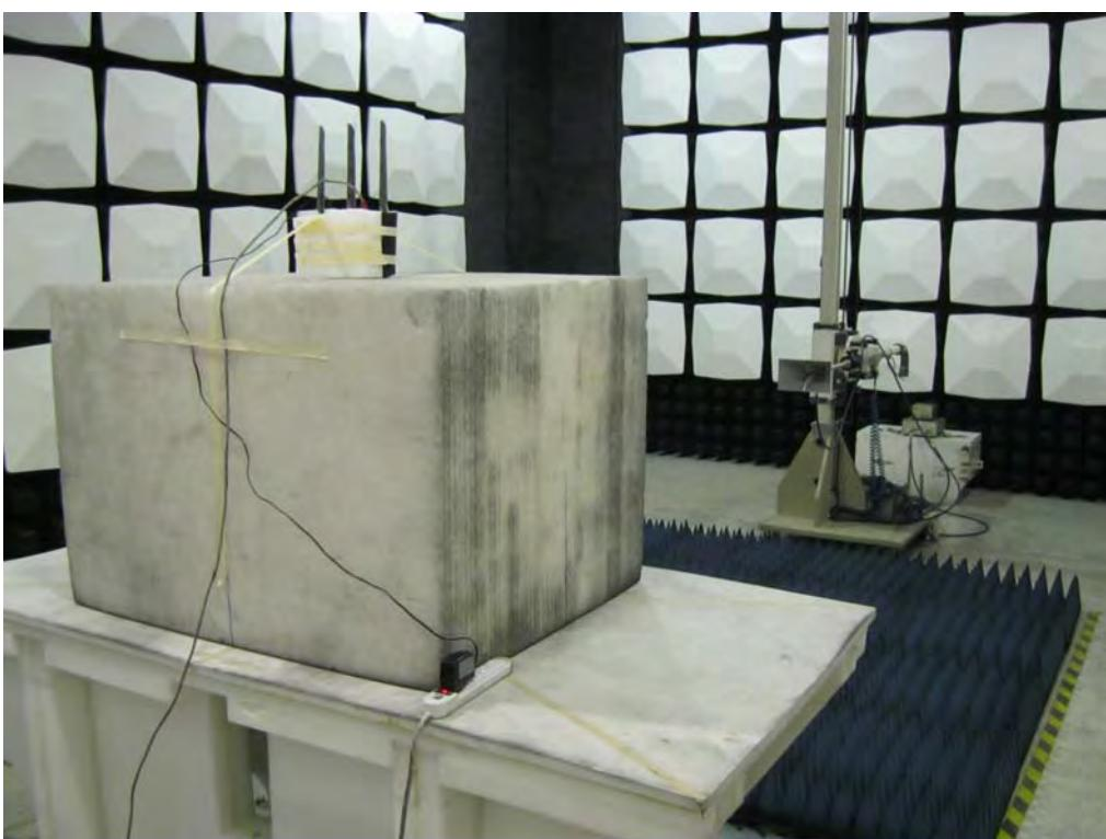
**ANTENNA PORT CONDUCTED RF MEASUREMENT SETUP**
