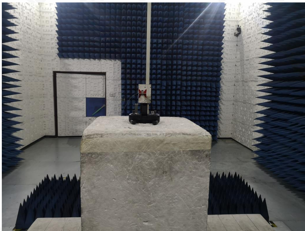
FCC RADIATED EMISSION TEST SETUP ABOVE 1GHZ
