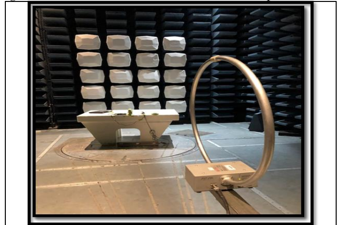
Figure R6: Radiated Emissions 30K-30M Hz Test Setup
