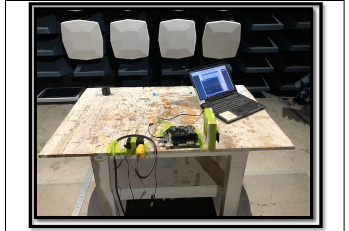
Figure R2: Radiated Emissions Test Setup w/ AE
