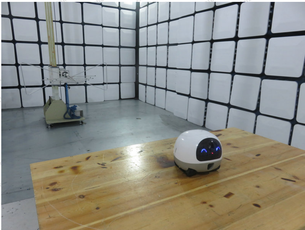
Photo of Radiation Emission Test
