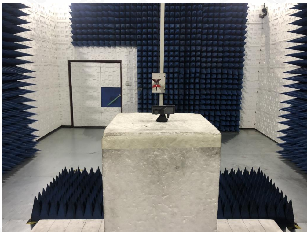
FCC RADIATED EMISSION TEST SETUP ABOVE 1GHZ
