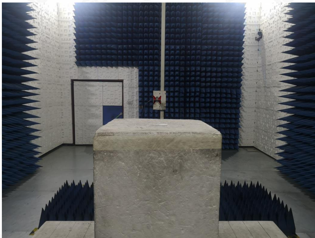
FCC RADIATED EMISSION TEST SETUP ABOVE 1GHZ
