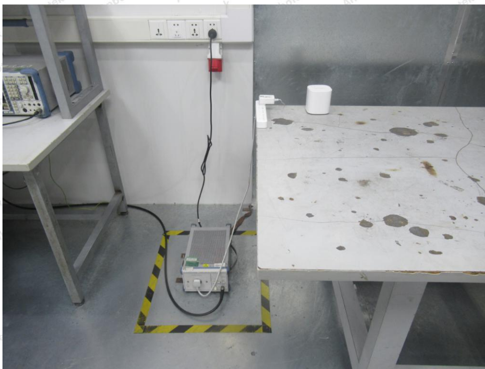
Photo of Power Line Conducted Emission Test
