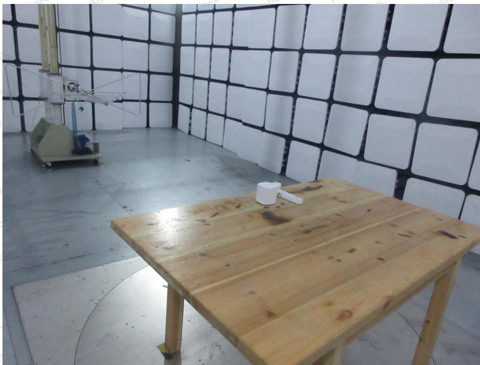
Photo of Radiation Emission Test
