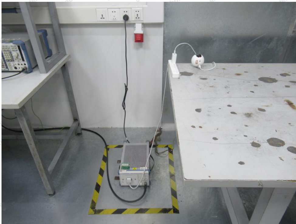
Photo of Power Line Conducted Emission Test
