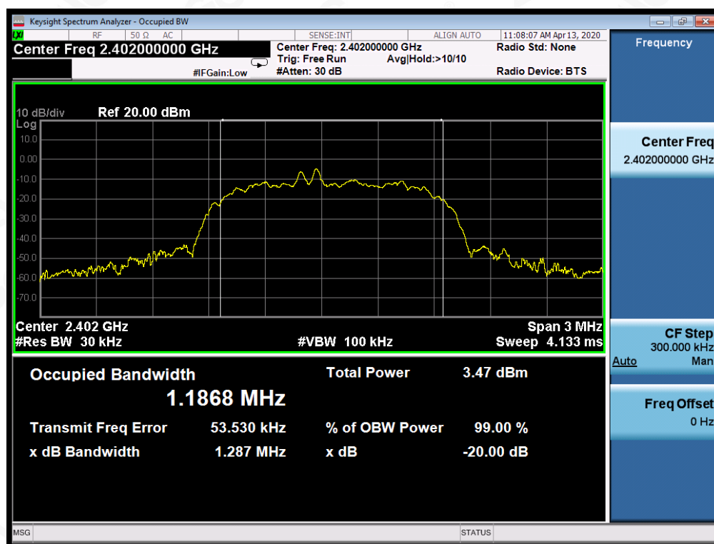
TEST PLOT OF BANDWIDTH FOR LOW CHANNEL
