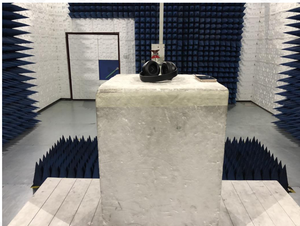
RADIATED EMISSION TEST SETUP ABOVE 1GHZ
