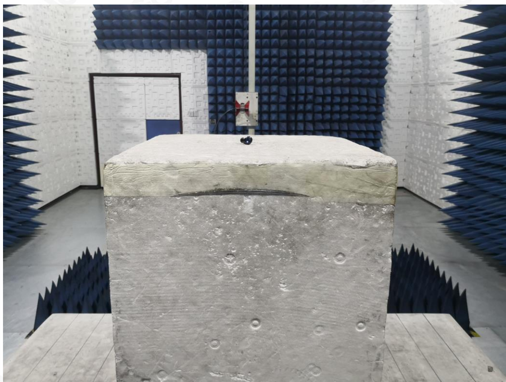
RADIATED EMISSION TEST SETUP ABOVE 1GHZ
