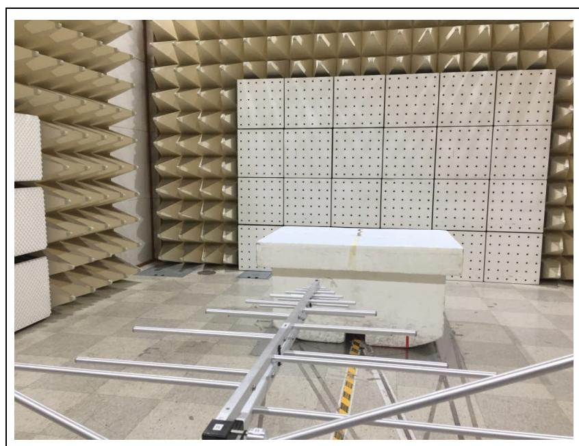
**3. Photo of Radiated Spurious Emission Test (Above 1 GHz)**
