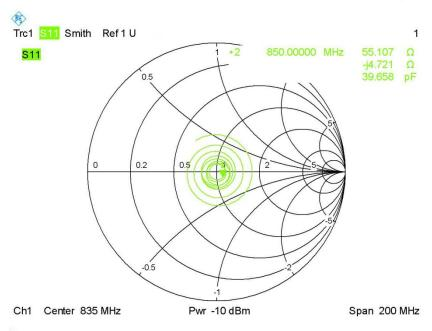
Calibrated return loss: -24.51dB; Measurement return loss: -24.34 dB(within 20%)
