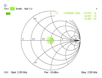
Calibrated return loss: -29.54dB; Measurement return loss: -29.55 dB(within 20%)
