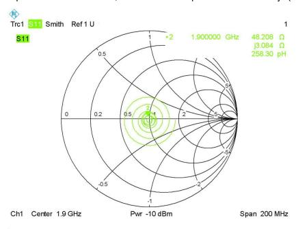
Calibrated return loss: -27.75dB; Measurement return loss: -28.32 dB(within 20%)
