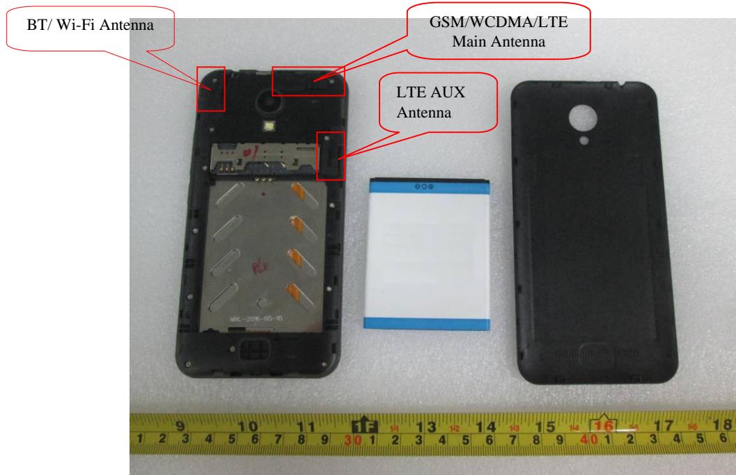
EUT – Cover off View 1
