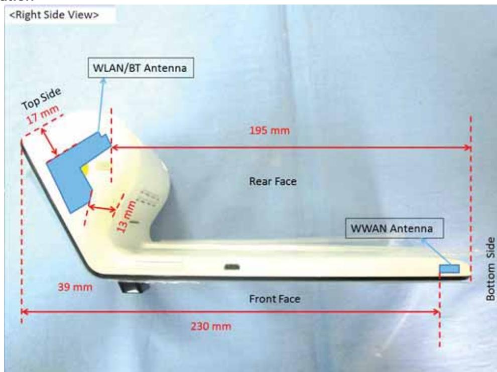
The separation distance for antenna to edge:
