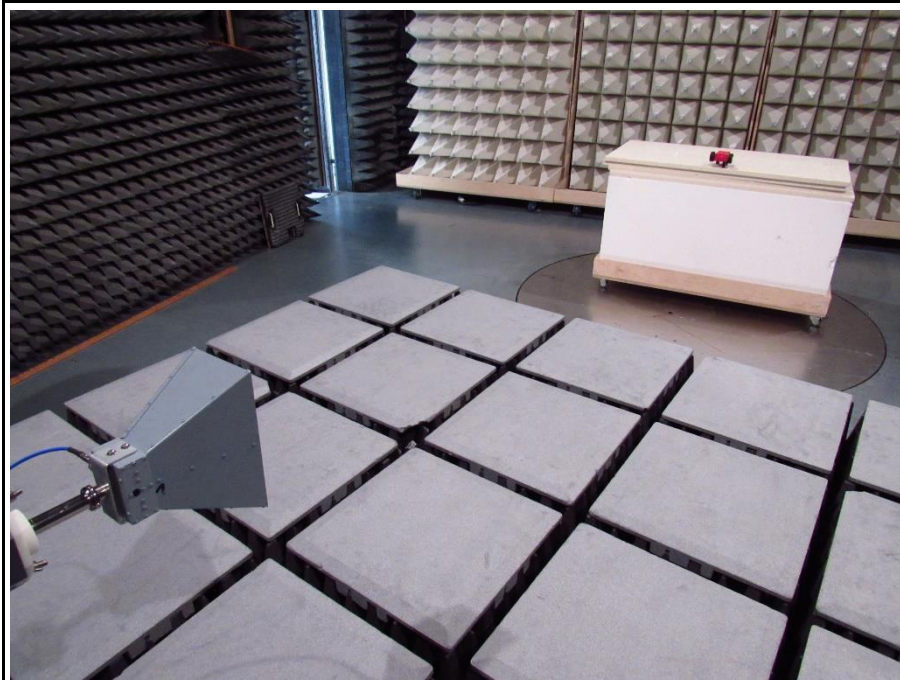
Test setup AC 1 0° position horizontal polarization up to 1 GHz
