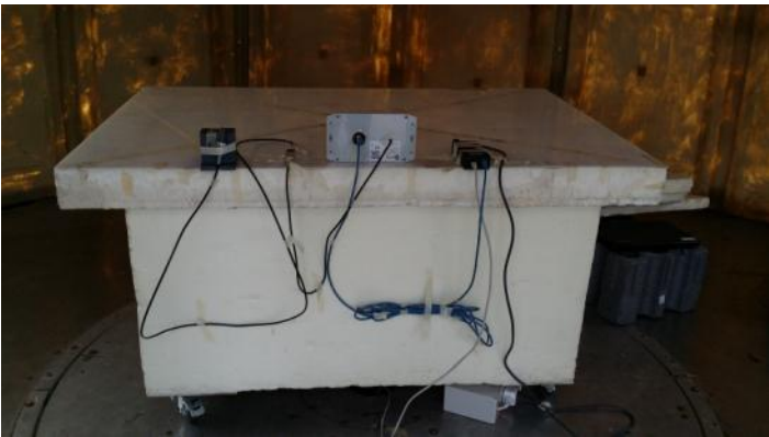
Test setup on OATS - §15.247 & §15.209 Configuration n°1 (Worst case)
