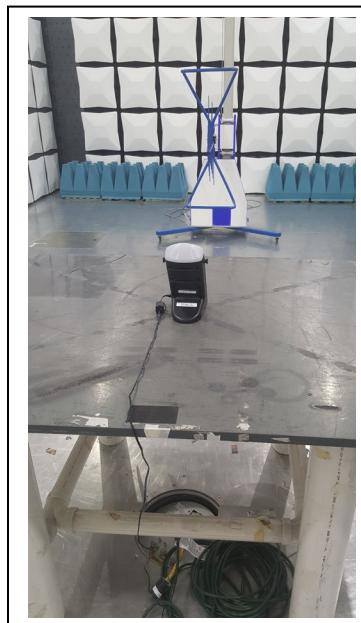
**Radiated Spurious Emission: 1 GHz to 10 GHz**
