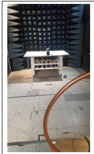
**Radiated Spurious Emission: 30 MHz to 1000 MHz**
