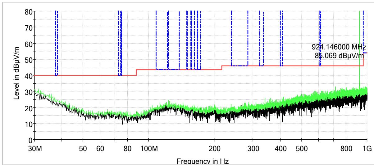
**QuasiPeak Measurements from all three channels.**
