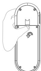
**Step 2:** Install 18650 battery and Mirco-SD.
