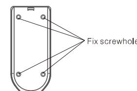
**Step 5:** Mount doorbell in the direction of the arrow and lock it by the screws at the bottom.
