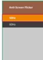
**Note:** Generally 60Hz is selected in the United States, Japan and other countries. In this way, the picture will not flicker because of the interference of the power frequency. It's usually 50Hz in Europe.
