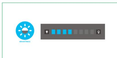
**Note:** The higher the brightness, the higher the power consumption.
