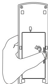
Step 2: Install 18650 battery and Mirco-SD.
