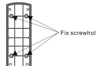
Step 5: Mount doorbell in the direction of the arrow and lock it by the screws at the bottom.
