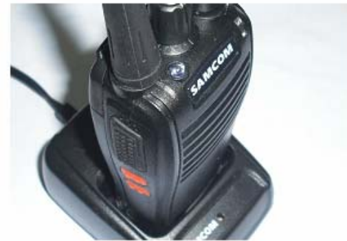
Set the Transceiver into the charger
