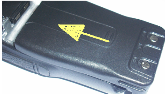
Install the battery pack
