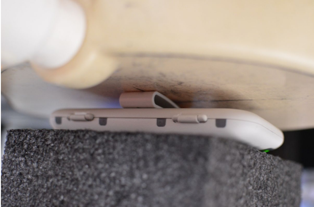
SAR Test Setup Photo 3: Body-worn – Back Side at 0 mm – with Clip
