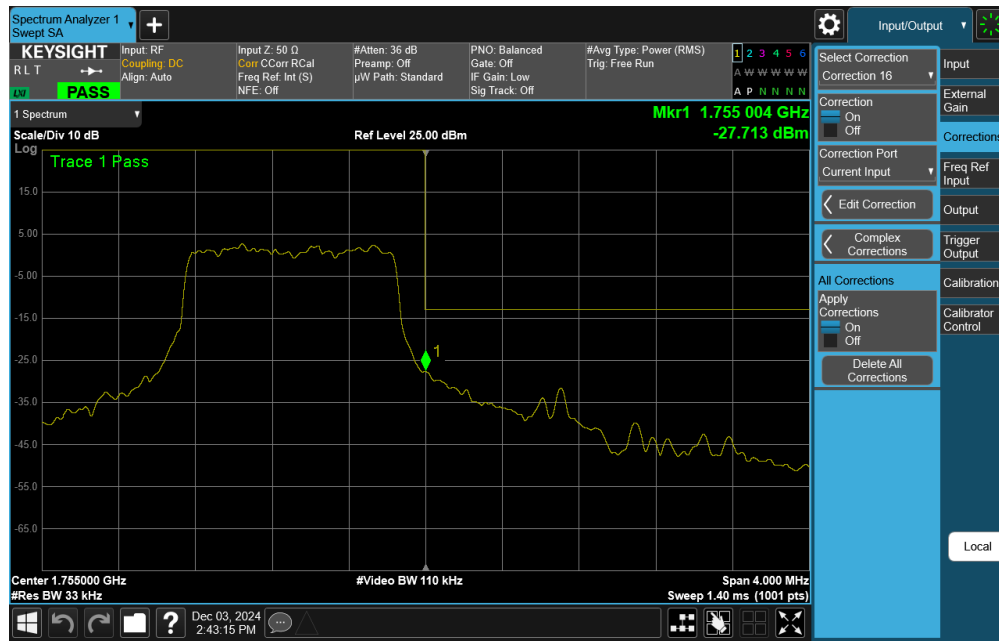
Plot 7-14. Upper Band Edge Plot (LTE Band 4 – 1.4MHz QPSK – Full RB)
