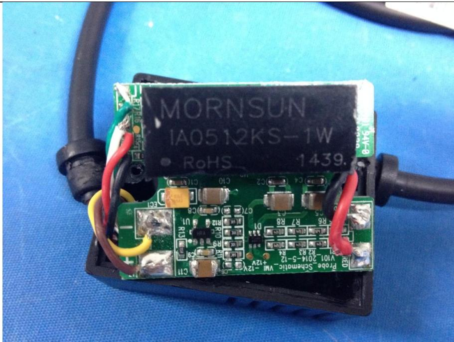
Details of: PCB Layout view 2 for Differential Probe
