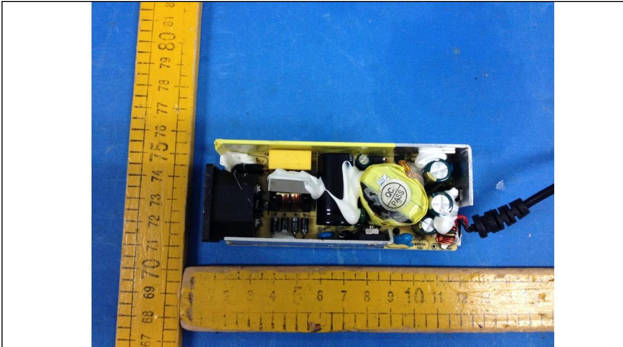
Details of: PCB Layout view 2 for AC/DC adaptor
