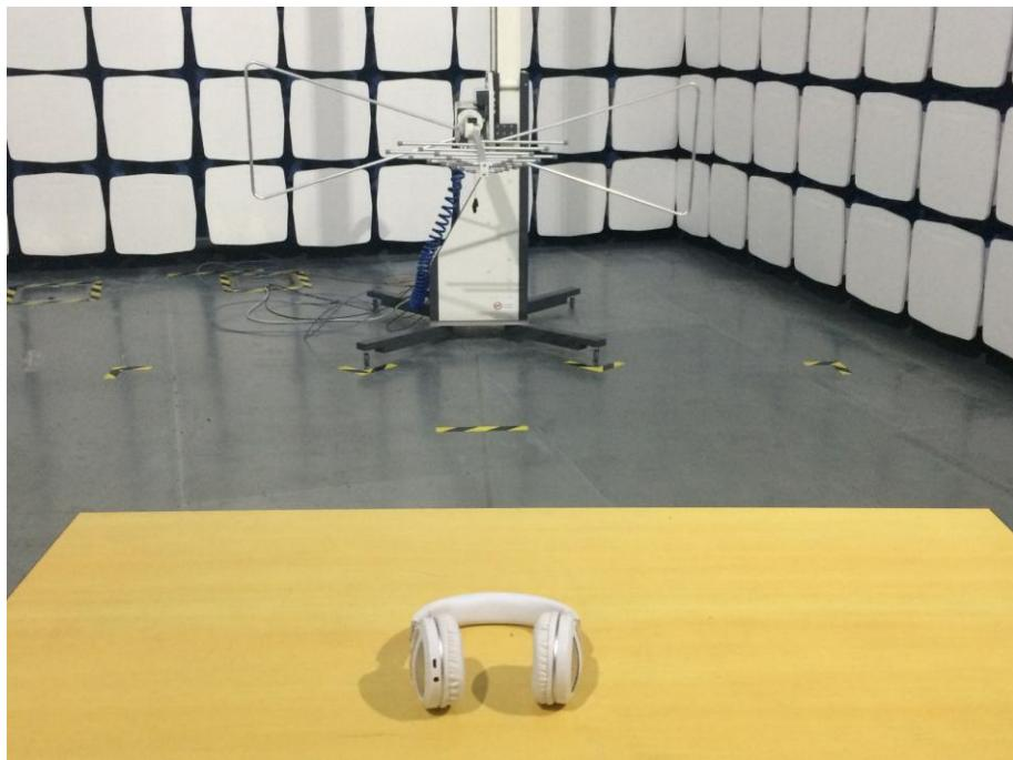
**Radiated Emission test view (Above 1GHz)**
