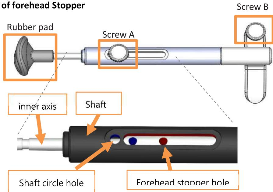
Step 1: Rolling the **inner axis** and the **shaft** to find out **forehead stopper hole**.
