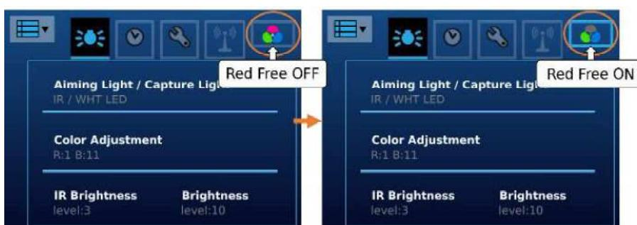
After turn on red free function, it will take more than 3 seconds to do image process after shooting. And there is a red free switch icon at the left-down corner of image. By press the icon to switch image into red free mode.
