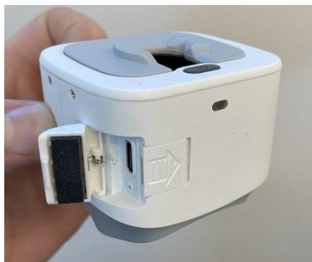
Charging port (door open)
