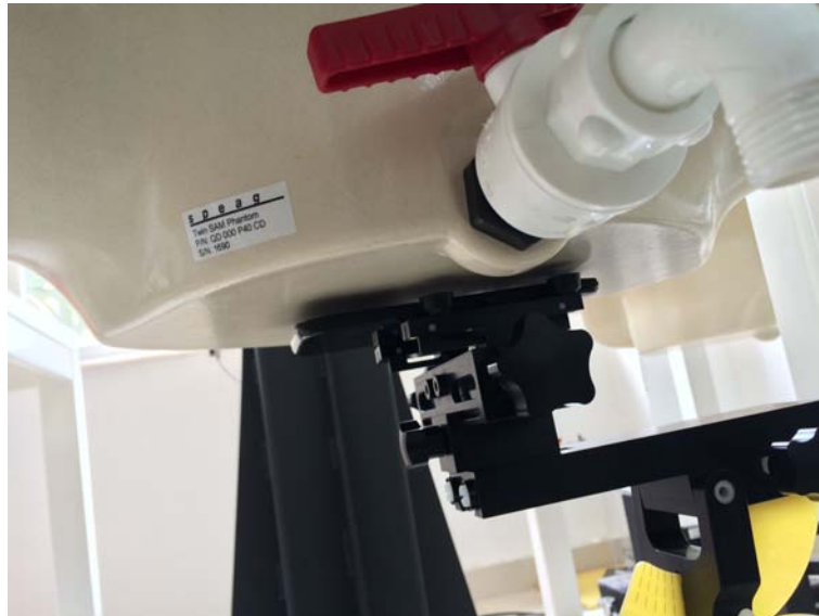
5mm Body-wornRear Side Setup Photo
