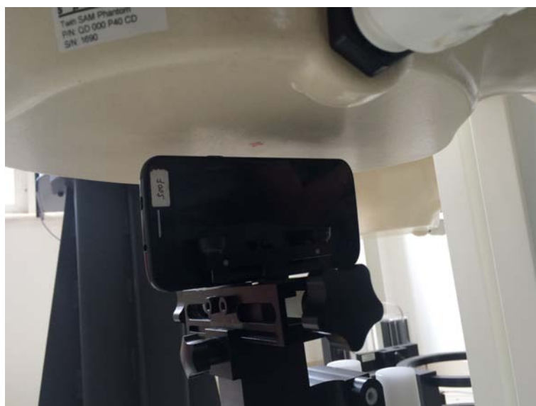
10mm hotspot Right Side Setup Photo
