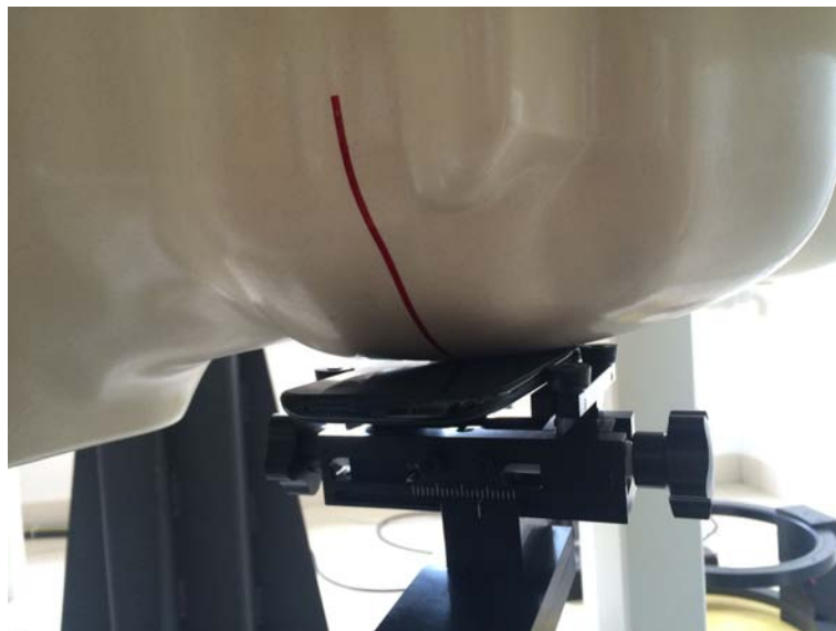
Left Head Cheek Setup Photo
