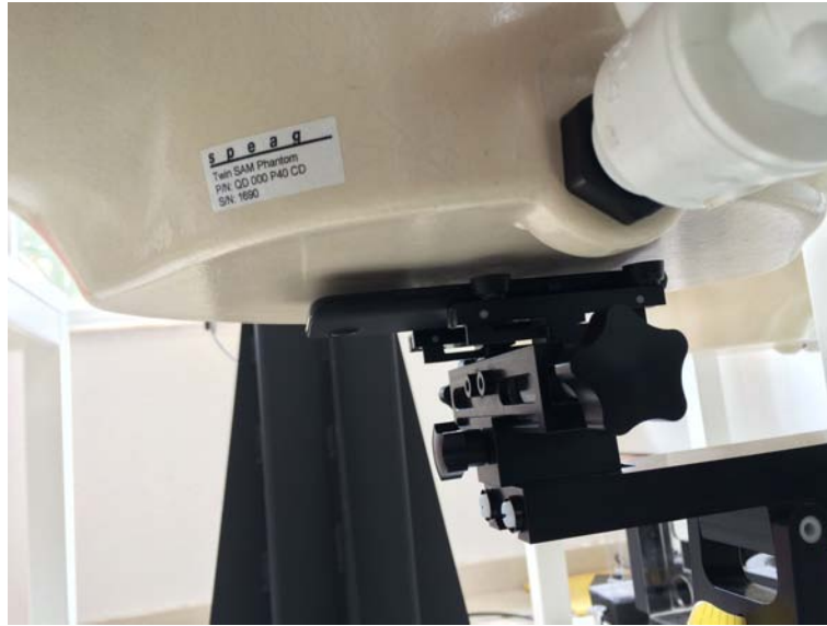
5mm Body-worn Front Side Setup Photo
