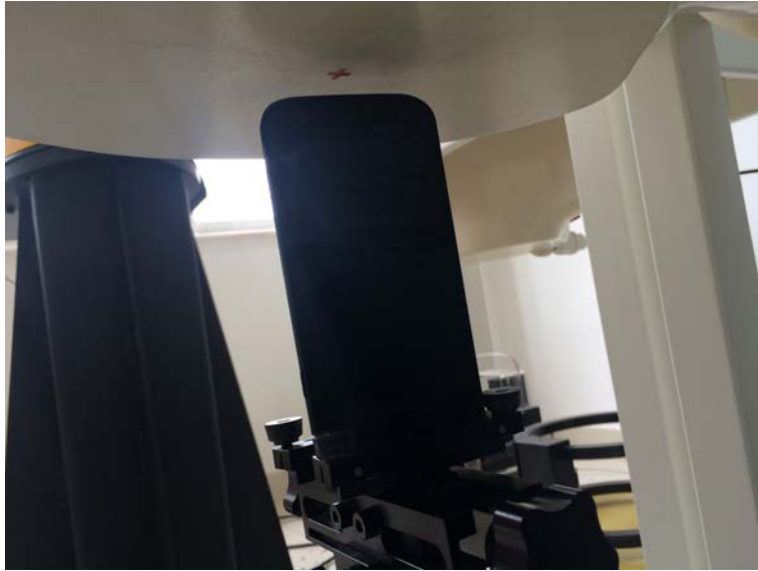
10mm hotspot Bottom Side Setup Photo
