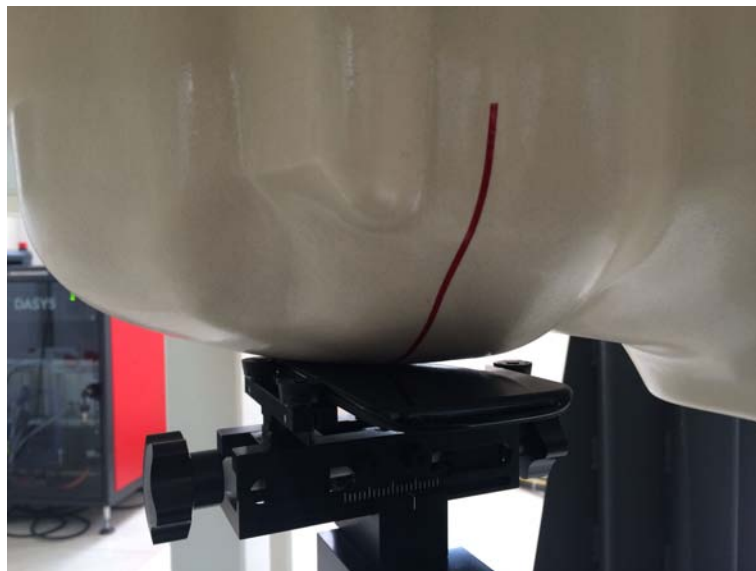
Right Head Cheek Setup Photo
