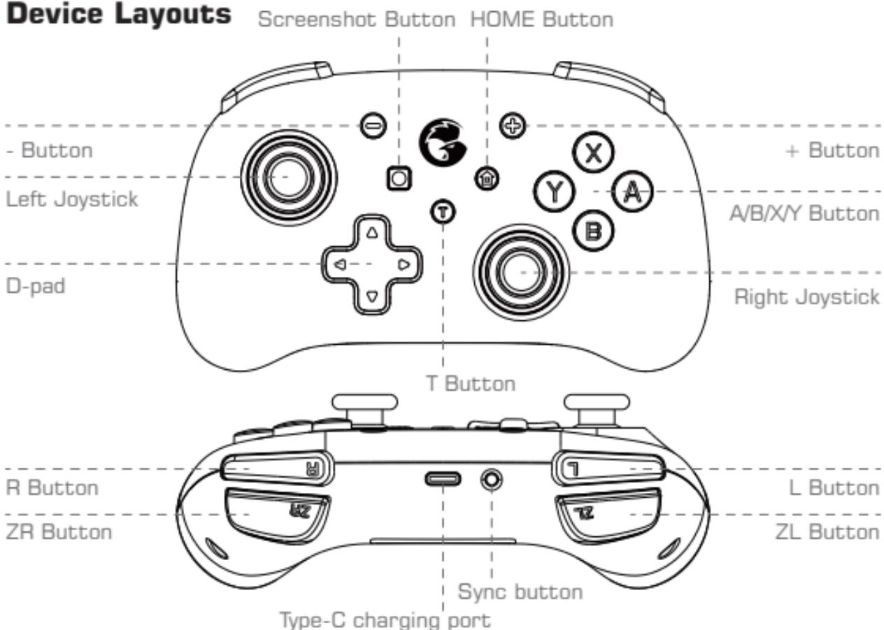
Power On: Press and hold the HOME button for 2s to power on;
