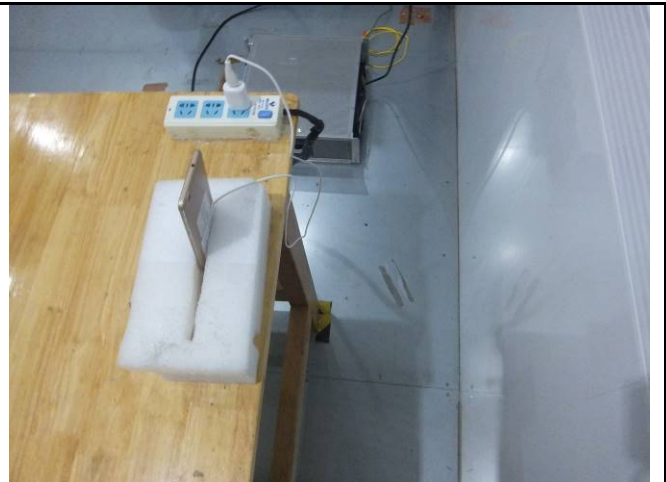
Conducted Emissions Test Setup Side View
