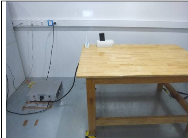
Conducted Emissions Test Setup Front View
