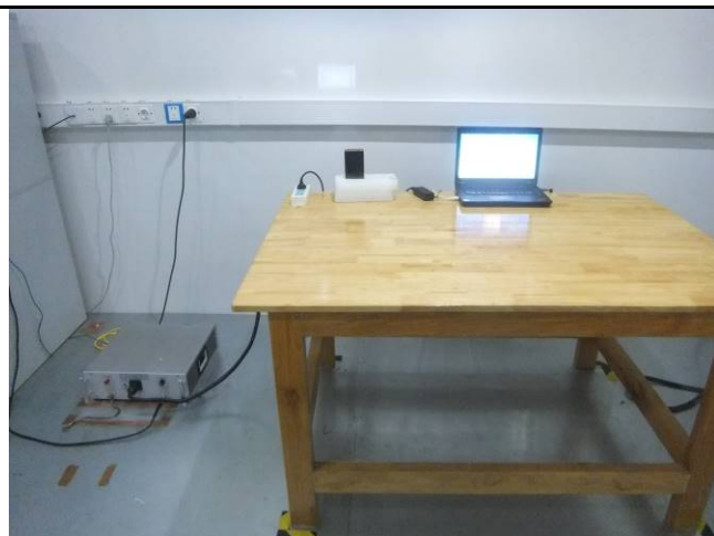
Conducted Emissions Test Setup – Front View
