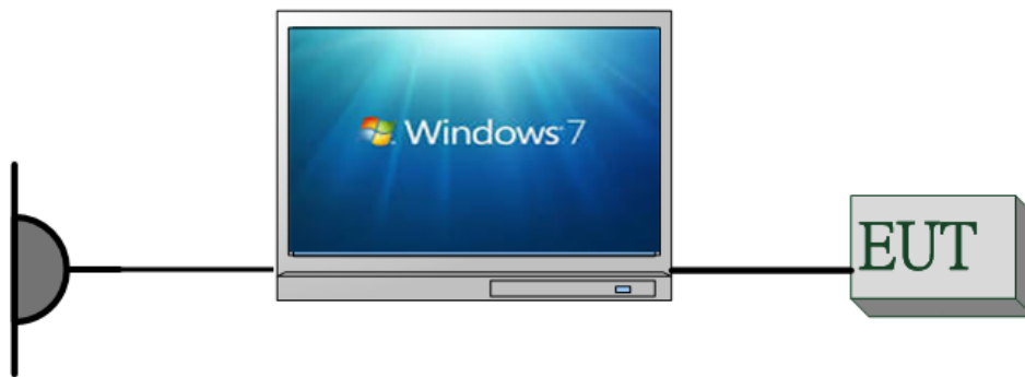
Fig. 2-1 Radiated Emission & Conducted (Antenna Port) Configuration
