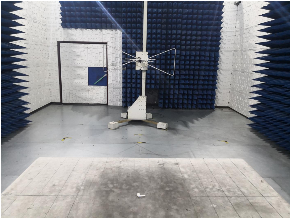
RADIATED EMISSION TEST SETUP ABOVE 1GHZ
