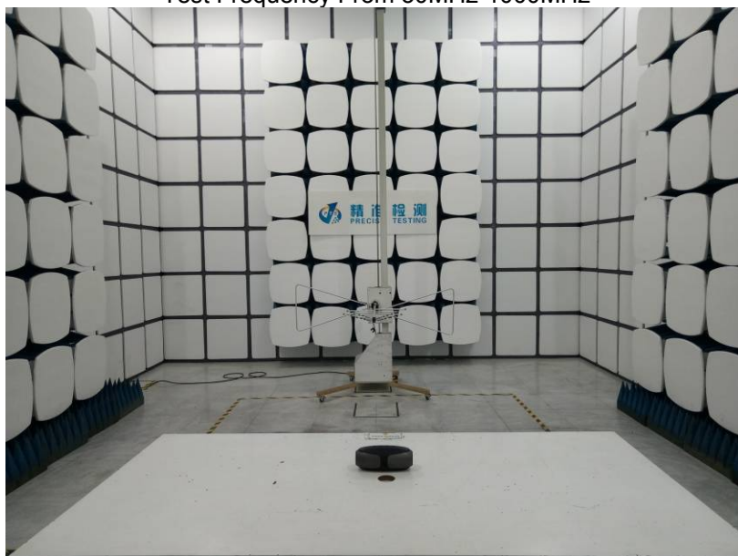
Radiated Spurious Emissions Test Frequency From 30MHz-1000MHz
