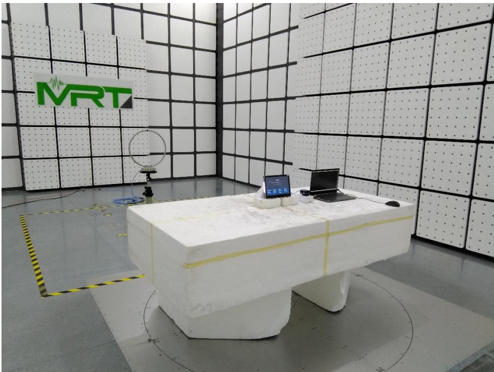
Description: Radiated Emission Test Setup for 9kHz~30MHz
