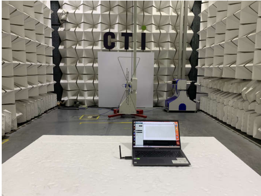
Radiated spurious emission Test Setup-1 (Below 1GHz)
