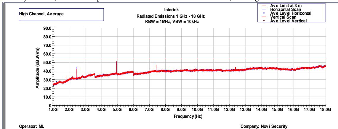
Note: Radiated emission measurements were performed up to 25GHz. No Emissions were identified when scanned from 18-25 GHz
