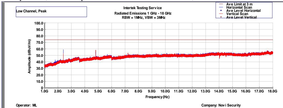
Novi Relay Station, Radiated Spurious Emissions 1000 - 18000 MHz, Average Scan
