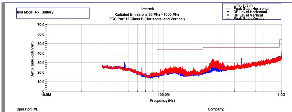
Test Results: Novi Sensor, Radiated Emissions 30 MHz – 1000MHz.
