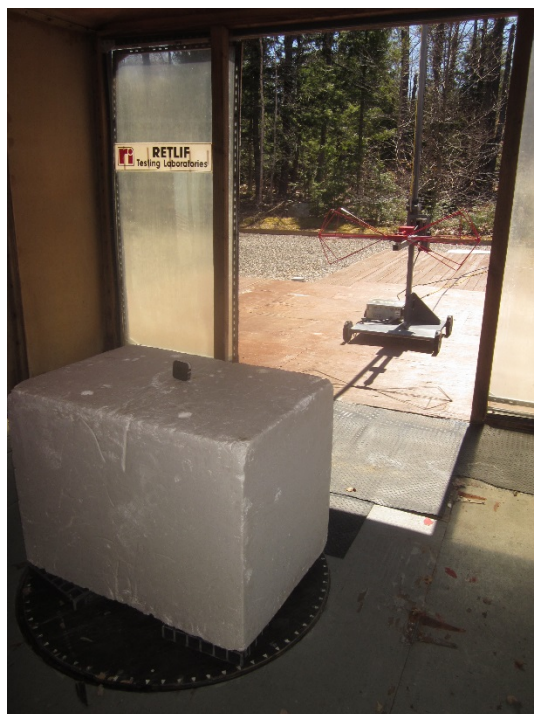
Horizontal Polarization, 30 to 200 MHz, Biconical Antenna, 80 cm
