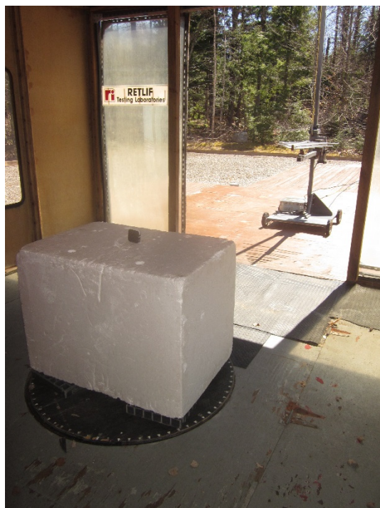
Horizontal Polarization, 200 MHz to 1 GHz, Log Periodic, 80 cm
