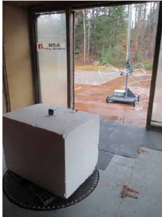
Horizontal Antenna Polarization, 30 to 200 MHz
