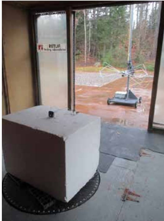
Horizontal Antenna Polarization, 30 to 200 MHz
