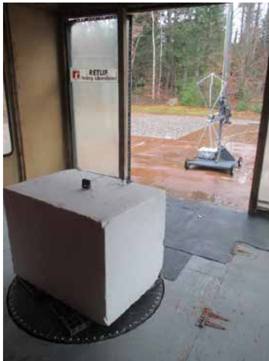
Vertical Antenna Polarization, 30 to 200 MHz
