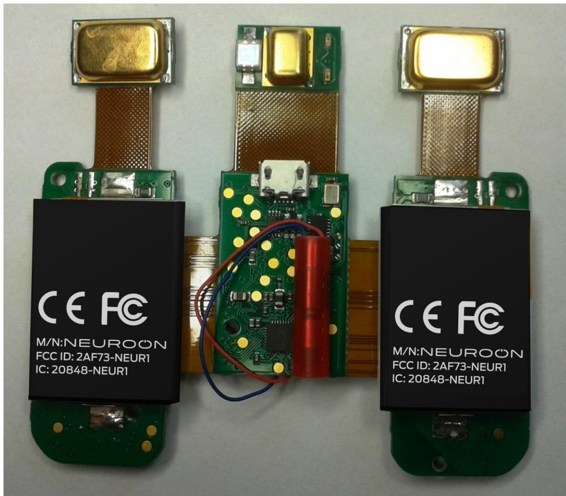
PCB without silicone potting, batteries, electrodes and vibration motor (facing away from the user):
